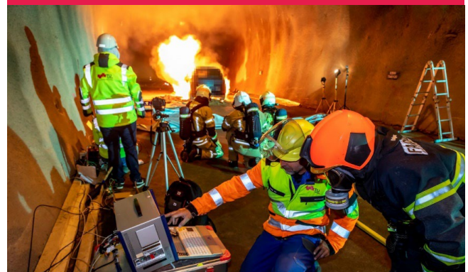
Graz University of Technology carries out fire tests of battery electric vehicles in summer 2021 © TU Graz/Lunghammer
