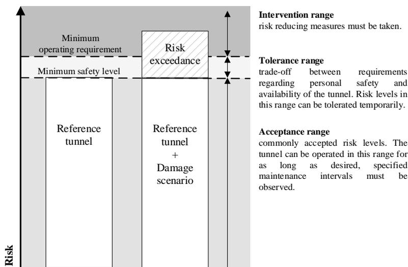
**Figure 2:** Thresholds of minimum safety level and minimum operating requirement dividing the risk axes into three ranges.
