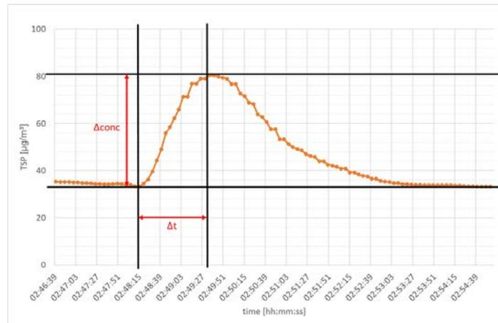
**Figure 6:** Concentration – time curve for a train passing the measurement location inside the tunnel
