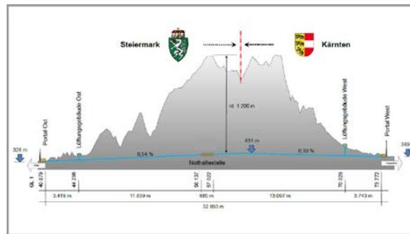
**Figure 2:** Longitudinal section of the Koralm Tunnel
