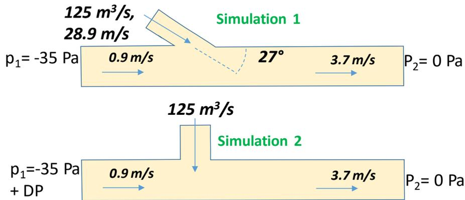
**Figure 10:** 3D Calculation conditions with Saccardo nozzles and with a vertical shaft
