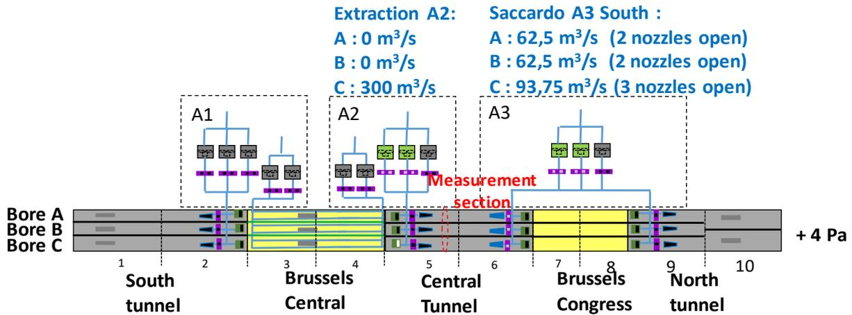
**Figure 11:** Ventilation scenario for a fire in section 5 – Bore C
