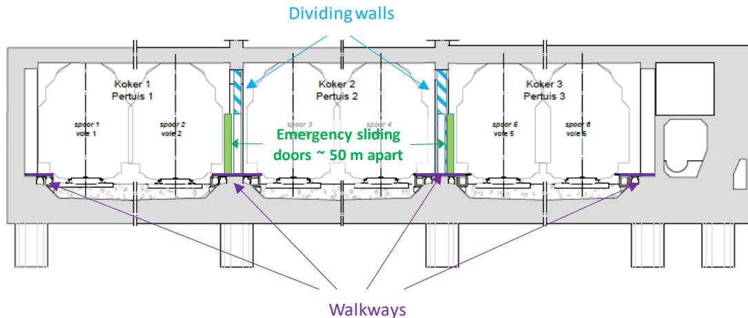
**Figure 2:** Typical tunnel cross-section after the refurbishment
