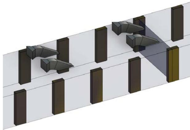
**Figure 9:** Saccardo nozzles and typical tunnel section of the North South Brussels junction
