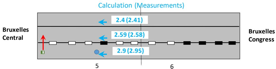
**Figure 12:** Comparison between measurements and cold smoke simulation with an efficiency of 0.81
