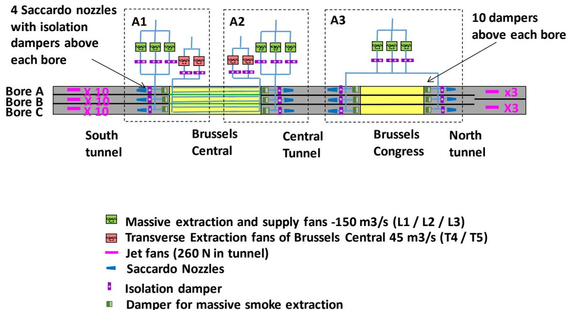
**Figure 5:** Synopsis of the ventilation system after refurbishment
