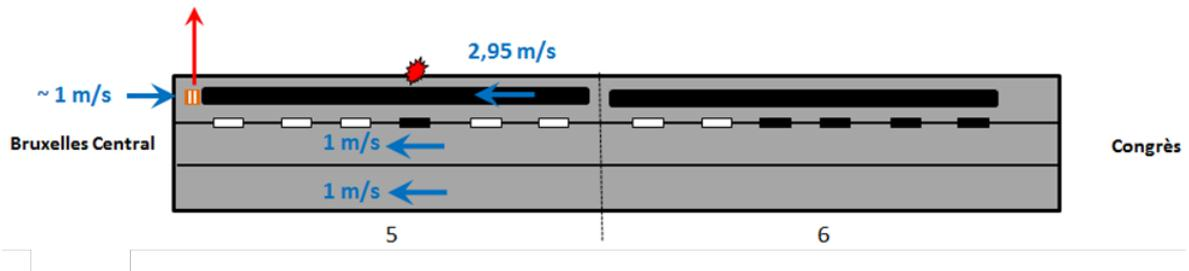
**Figure 4:** Objectives of tunnel emergency ventilation
