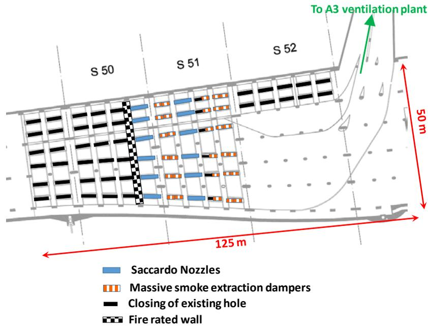
**Figure 7:** Ventilation plenum of A3 South – Plan view
