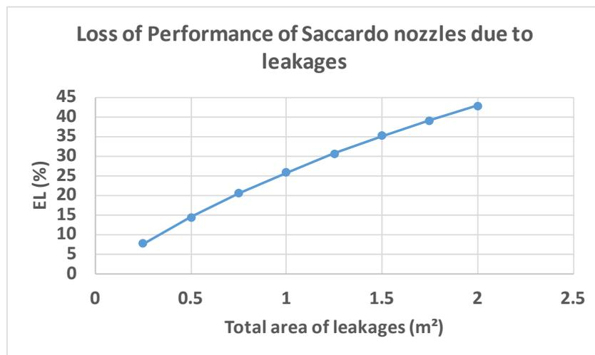
**Figure 8:** Loss of efficiency of Saccardo nozzles due to leakages
