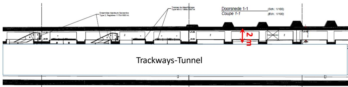
Figure 6: Ventilation plenum of A3 South –Elevated view
