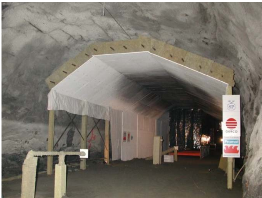
Figure 2: Fire protection of the Runehammar test tunnel shown from the east (upstream) side and the HGV trailer mock-up (Ingason, Lönnemark, & Li, 2011).
