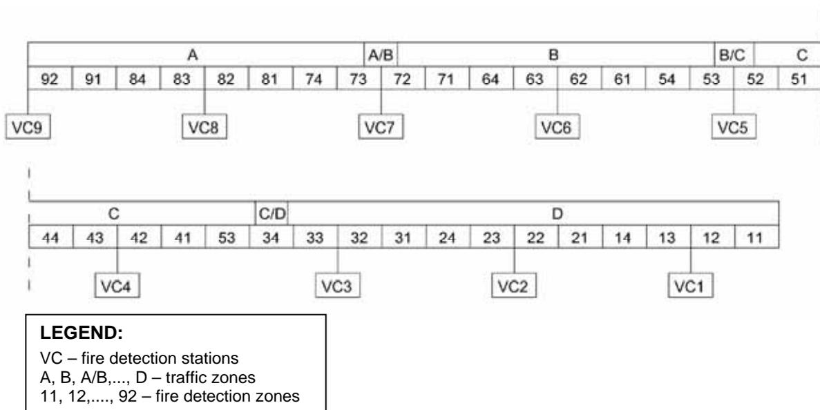
**Figure 4:** Schematic presentation of the fire alarm system
