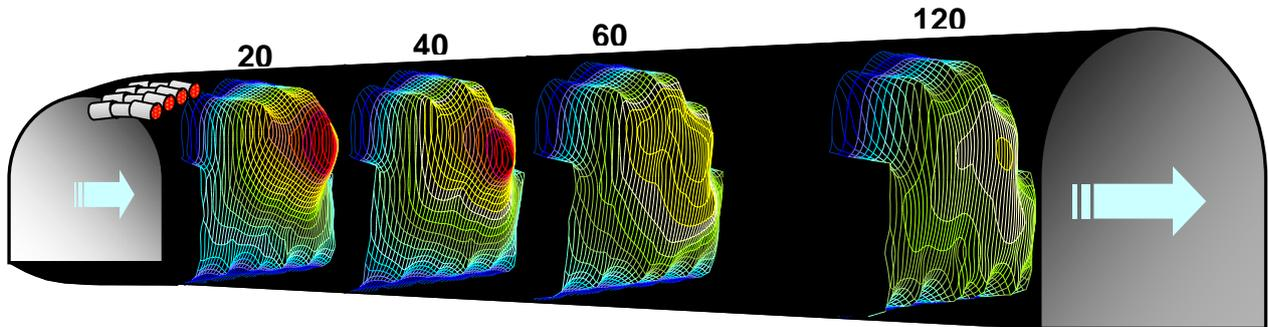
**Figure 6: Air speed profile across the tunnel cross section of Uznaberg West tunnel Banana Jet**
