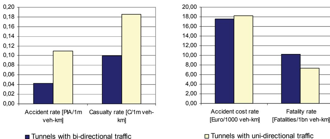
**Figure 2:** Relative accident rate for tunnels with bi-directional traffic and unidirectional traffic (1999-2007)
