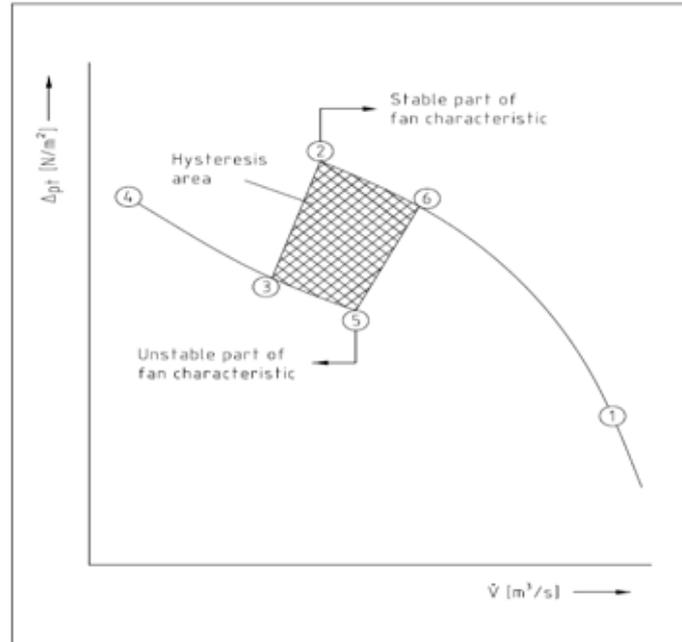
**Figure 2:** Typical performance graph axial flow fan at fix rotor blade angle and at constant speed
