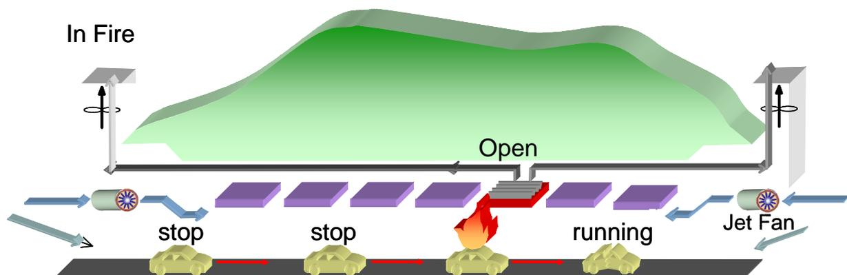
**Figure 2-6:** Point extraction system in the case of fire
