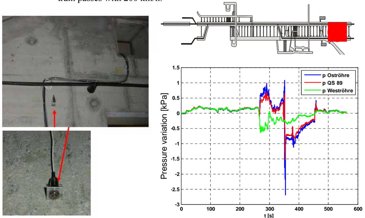
**Figure 5:** Train induced pressure loads in the south eastern and western railway tubes and in the cross passage between the two single track railway tubes while passing of a passenger train (ICE,  $V_{max}=200$  km/h). On the left side: Installed pressure sensors. On the upper right side: Localisation of the measurement. On the lower right side: Measured data
