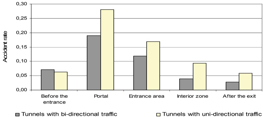
**Figure 4:** Personal injury accident rate [PIA/1 million vehicle-kilometres] in tunnels with bi-directional traffic and unidirectional traffic by point of origin of the accident (1999-2007)
