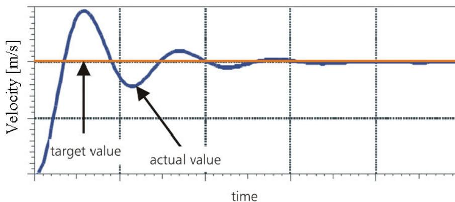
**Figure 4:** Behaviour in case of a closed loop control
