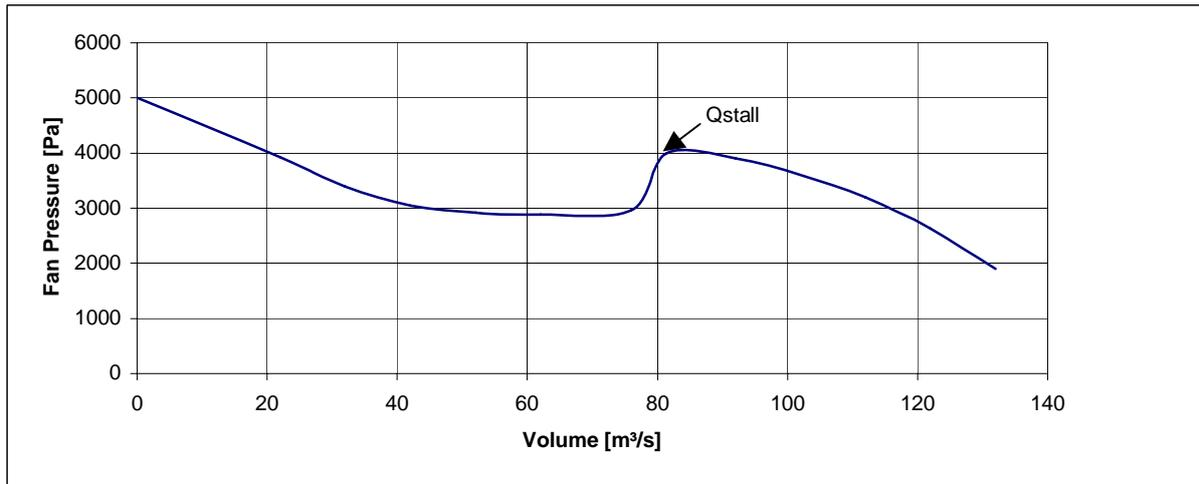
**Figure 1: Fan curve fixed pitch fan**
