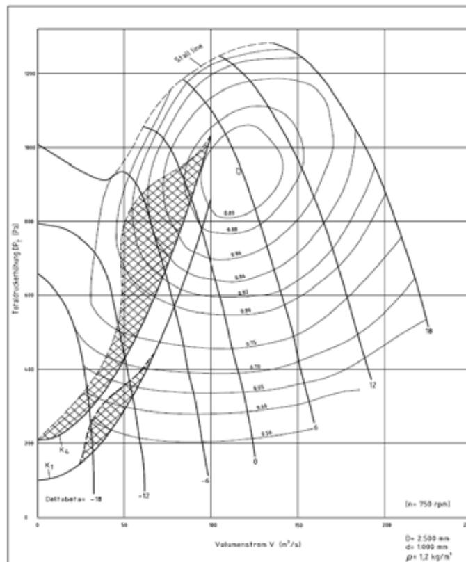
**Figure 7:** Fan performance chart with systems resistance characteristics  $K_1$  and  $K_4$
