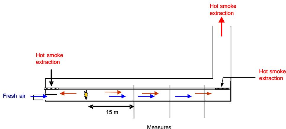
**Figure 2** : Experimental set-up for smoke stratified layer characterisation.
