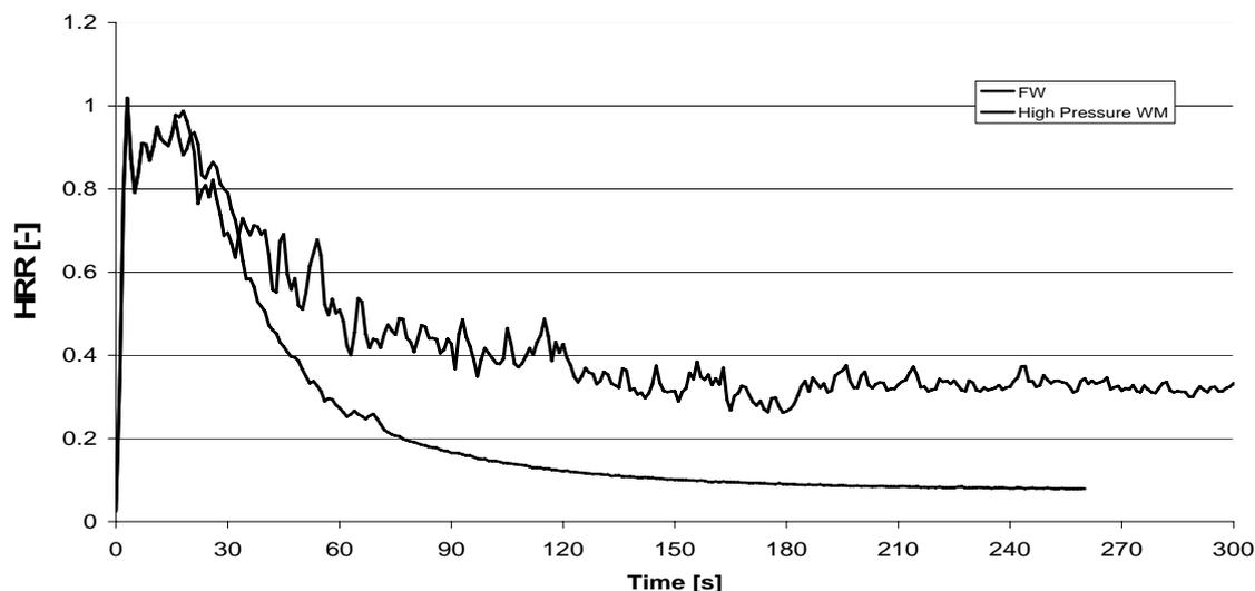
**Figure 1:** Test results from Foam Water and high pressure Water Mist systems to a 50MW fire.
