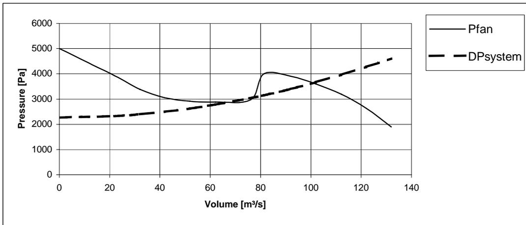
Figure 5: System resistance line and fixed pitch fan curve
