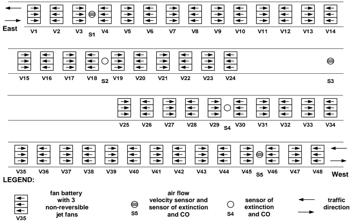
**Figure 2:** Schematic presentation of the arrangement of jet fan batteries, air flow velocity sensors and sensors of extinction and CO
