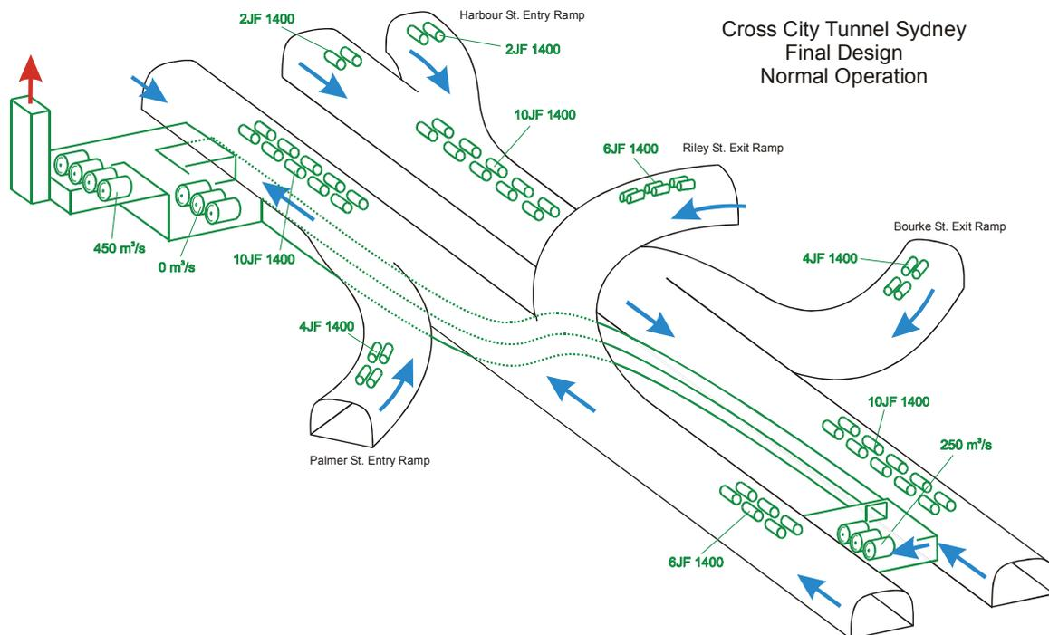
**Figure 8:** Cross-City Tunnel (Sydney, Australia). The capacity of the ventilation system is: cross-ventilation station 250 m<sup>3</sup>/s; bypass-ventilation station 340 m<sup>3</sup>/s, exhaust-ventilation station 690 m<sup>3</sup>/s and 54 jet fans each with a static thrust of 1650 N.
