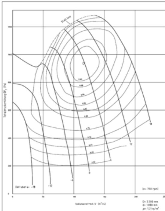
**Figure 3:** Fan performance chart for variable rotor blade adjustment during operation
