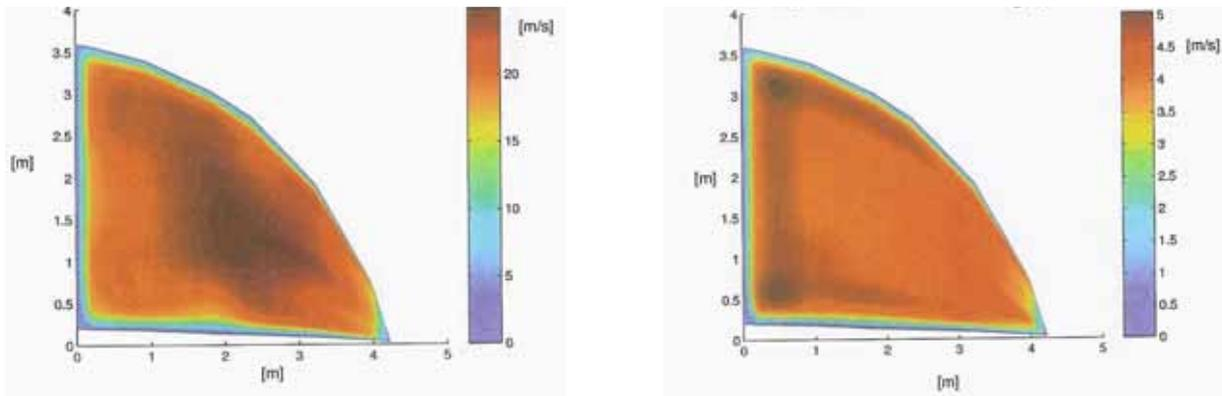
**Figure 3:** Velocity profiles in the tunnel (left) and close to the ventilation station Airolò (right). The peculiar shape of the second profile is related to the tunnel's curvature in the portal area (radius 760 m).
