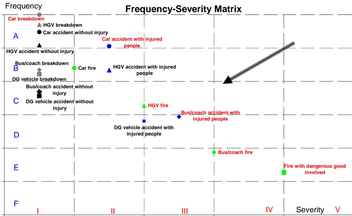
**Figure 2:** Frequency – Severity Matrix, according to [4]
