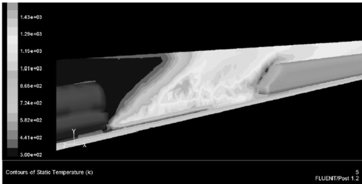
**Figure 7:** simulation of a major fire next to a passenger train
