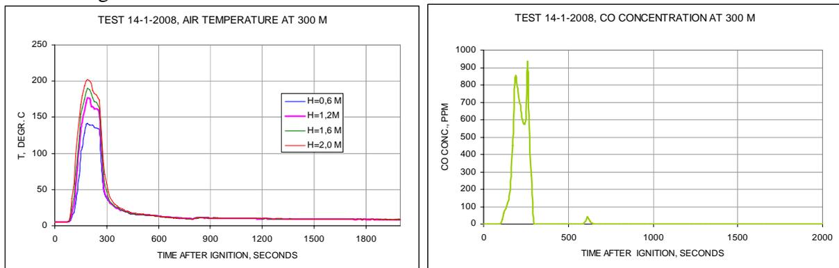
**Figure 13:** This sample shows the data recorded during performance test 2, at 300 m
