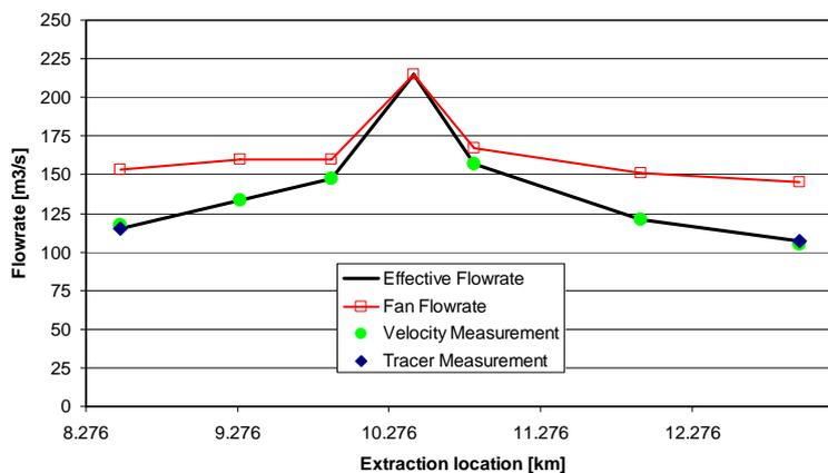
**Figure 6:** Leakages measured in the Branisko Tunnel.
