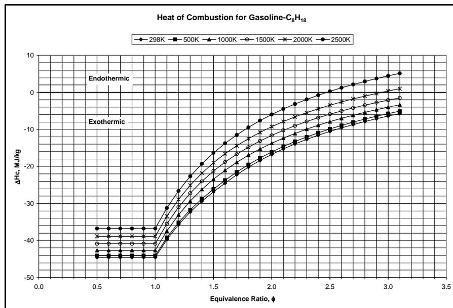
**Figure 1:** Heat of combustion for gasoline as a function of  $\phi$  and temperature
