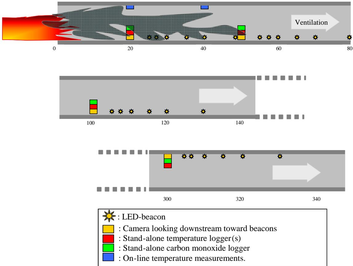
**Figure 12:** The physical layout and position of the cameras and sensors used to measure tenability. Each camera looks at six beacons, set at distances of 5, 7, 10, 15, 20 and 30 m.
