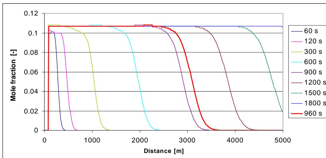
**Figure 5:** Dispersion after a leak (50mm) of ammonia (taken ventilation speed 3 m/s).
