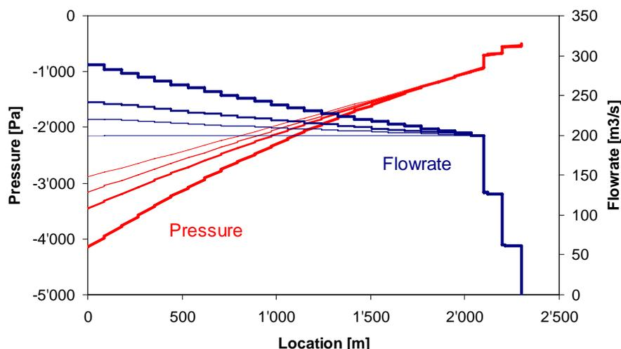
**Figure 1:** Flow rate and pressure distribution in case of fire for different leakage rates (Gotthard road tunnel, southernmost ventilation section, Airolo-Motto di Dentro). The curves indicate the results obtained imposing a constant extraction rate of 200 m<sup>3</sup>/s through 3 open dampers with high (thickest lines), average and vanishing leakage rates (thinnest lines). The leakage rates correspond to the prescriptions of the Swiss directive as well as half resp. twice this value.
