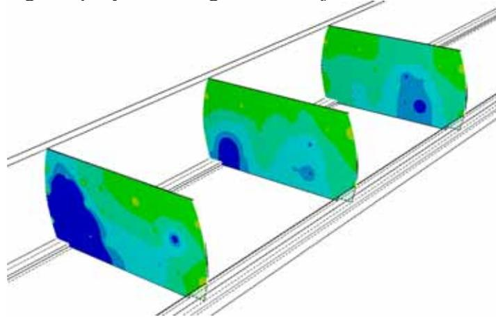
**Figure 3:** Result for water spray distribution in the cross section
