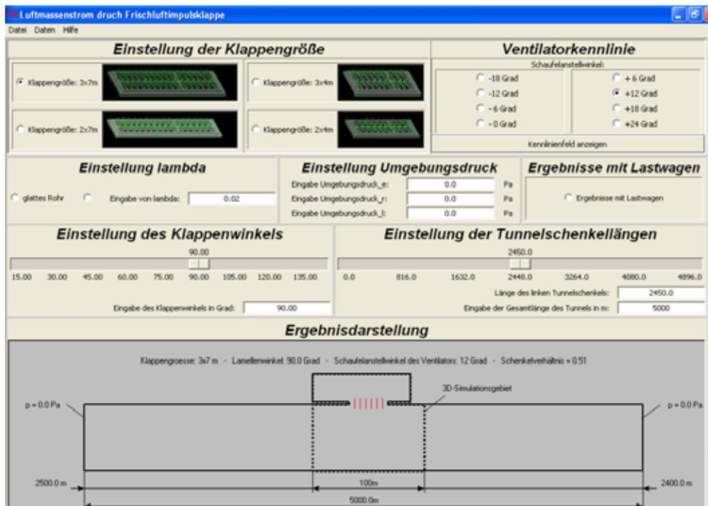
**Figure 1:** Working surface of the selection software
