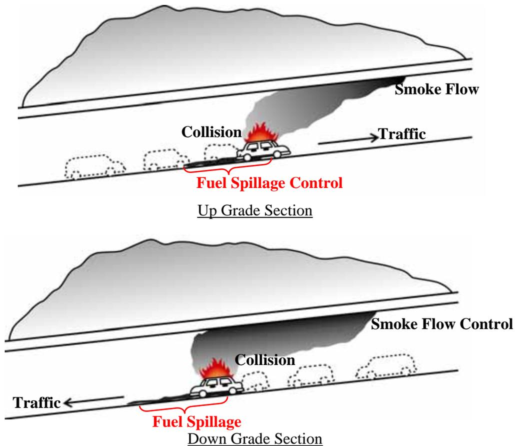
**Figure 2-2:** Basic concept for the safety design in grade section
