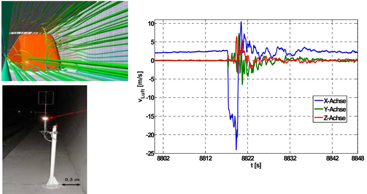
**Figure 4:** Three dimensional air flow in the railway tunnel. On the upper left side: An illustrative 3D simulation of turbulent air flow along a moving high speed train in the tunnel. On the lower left side: The used ultra sonic air speed sensors to capture the three dimensional air flow in the railway tube. On the right side: Measured 3D air flow on the sideway in the railway tube while a passenger train passes with 200 km/h.
