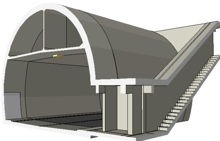
**Figure 2:** Felbertauerntunnel escape route system diagram
