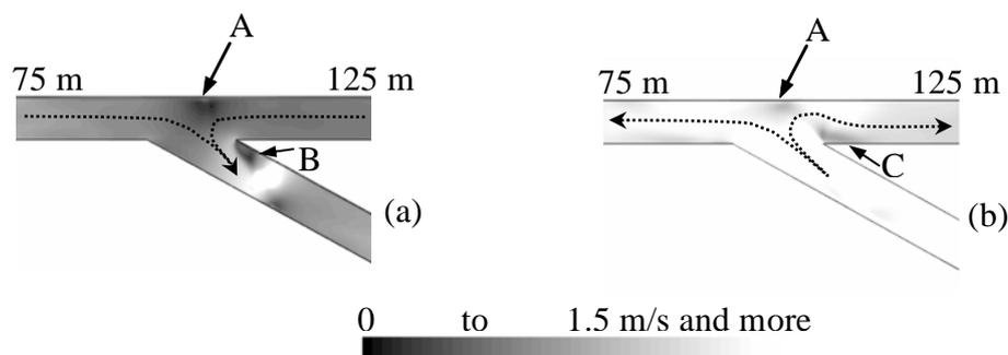
**Figure 3:** The velocity field in the air, when the fire is in the lateral branch
