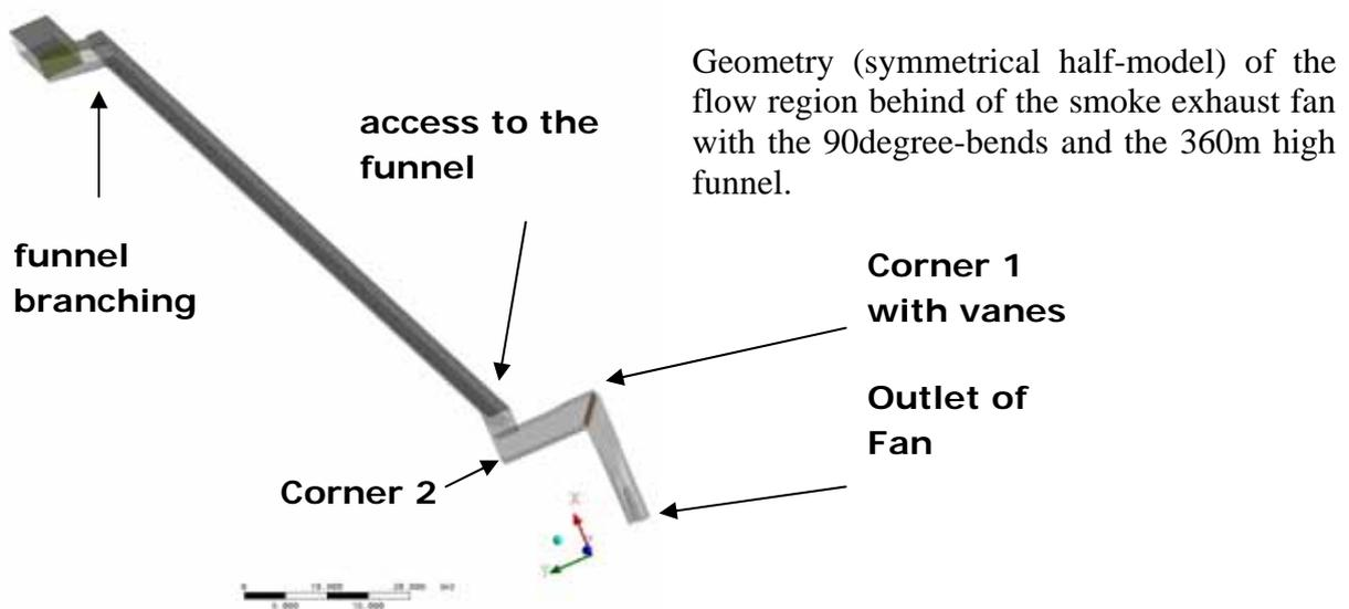
Fig. 1.: Geometry of the flow region behing smoke exhaust fan
