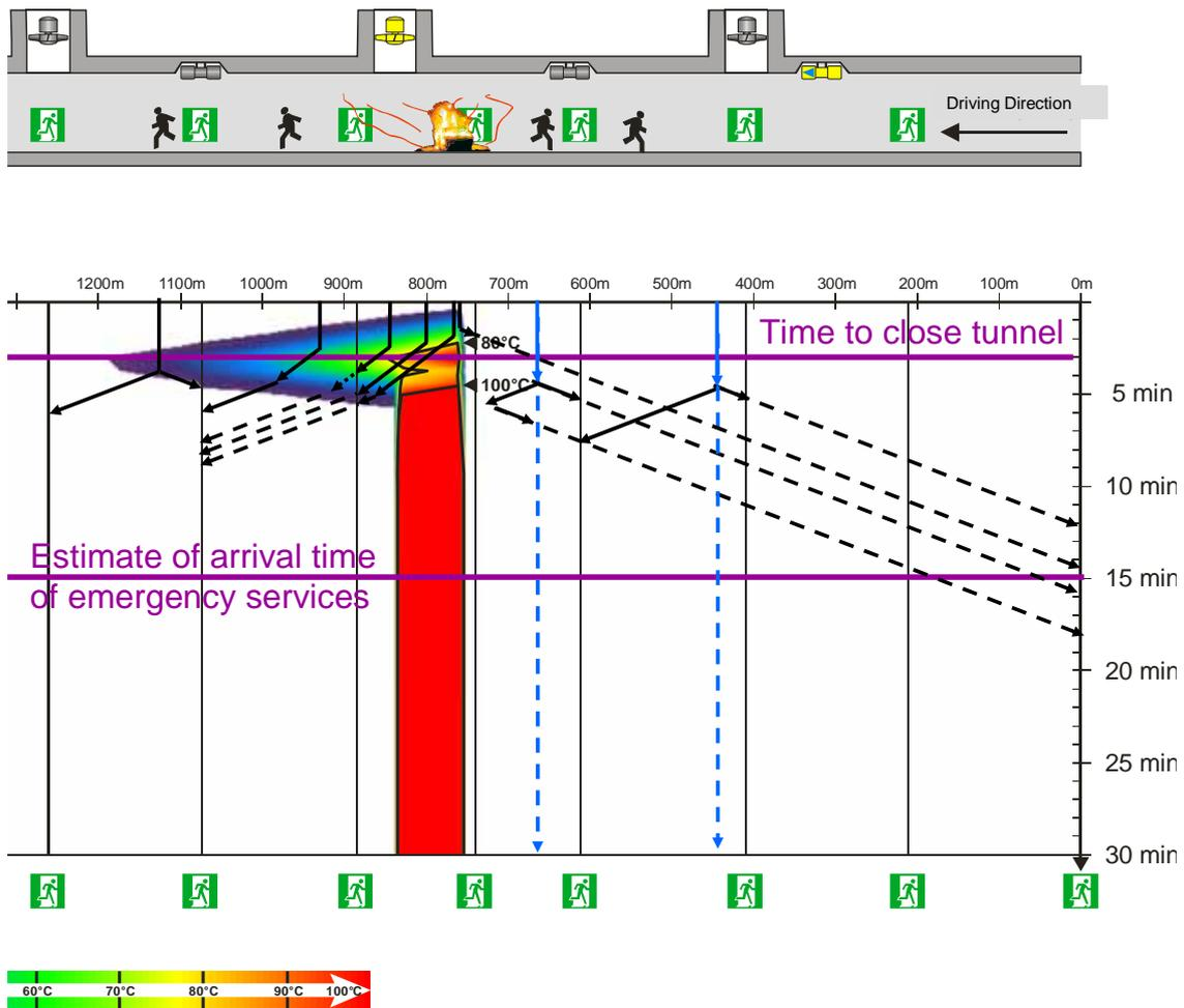
**Figure 3:** Representation of consequences for people of a fire in tunnel
