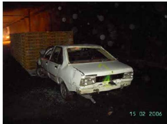
**Figure 1+2:** Fuel package (real car + 2 x 12 x 9 pallets on the floor level + target cars)
