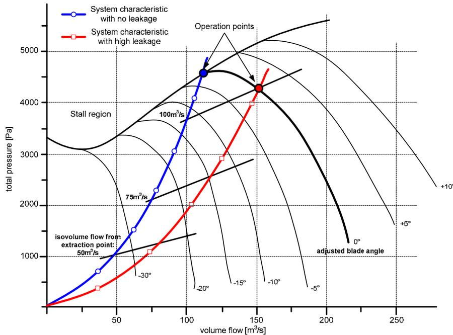
**Figure 1:** System characteristics regarding leakage
