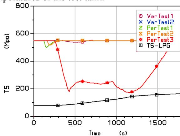
**Figure 11:** Maximum stress that the wall can withstand for each test versus the actual stress (label TS-LPG) in PerTest3. Note: the actual stress in the other tests is lower than in “PerTest3”.
