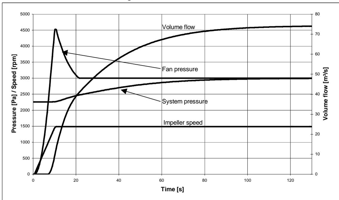
Figure 6: Start-up second fan with fixed pitch system
