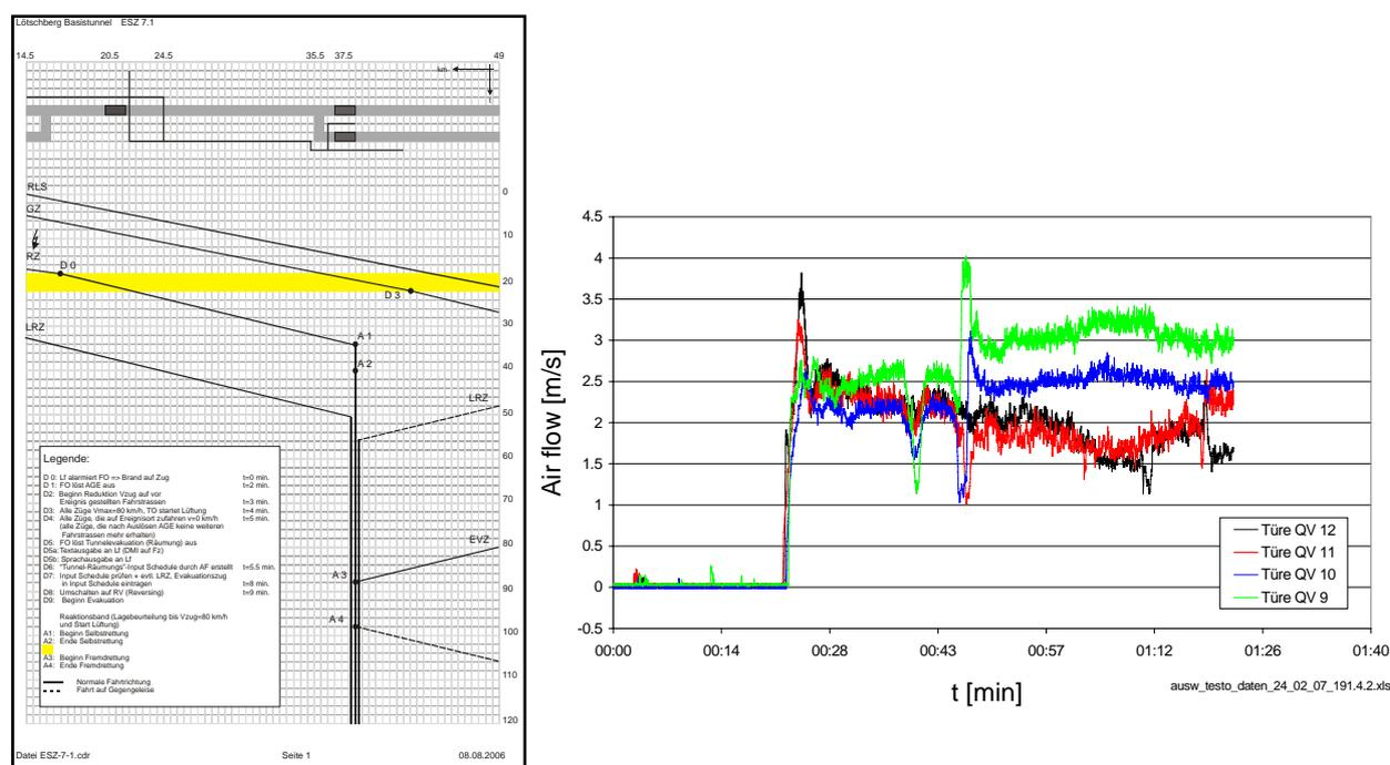
**Figure 8:** Tests of the emergency ventilation system: On the left side: Typical emergency operation scenario in the tunnel based on the train control system ETCS II. On the right side: Measured longitudinal air speed in the open escape doors of the rescue station as a result of the supplied fresh air of the emergency ventilation system. The temporal fluctuation of the air flow bases on the piston effect of the train movements in the tunnel.
