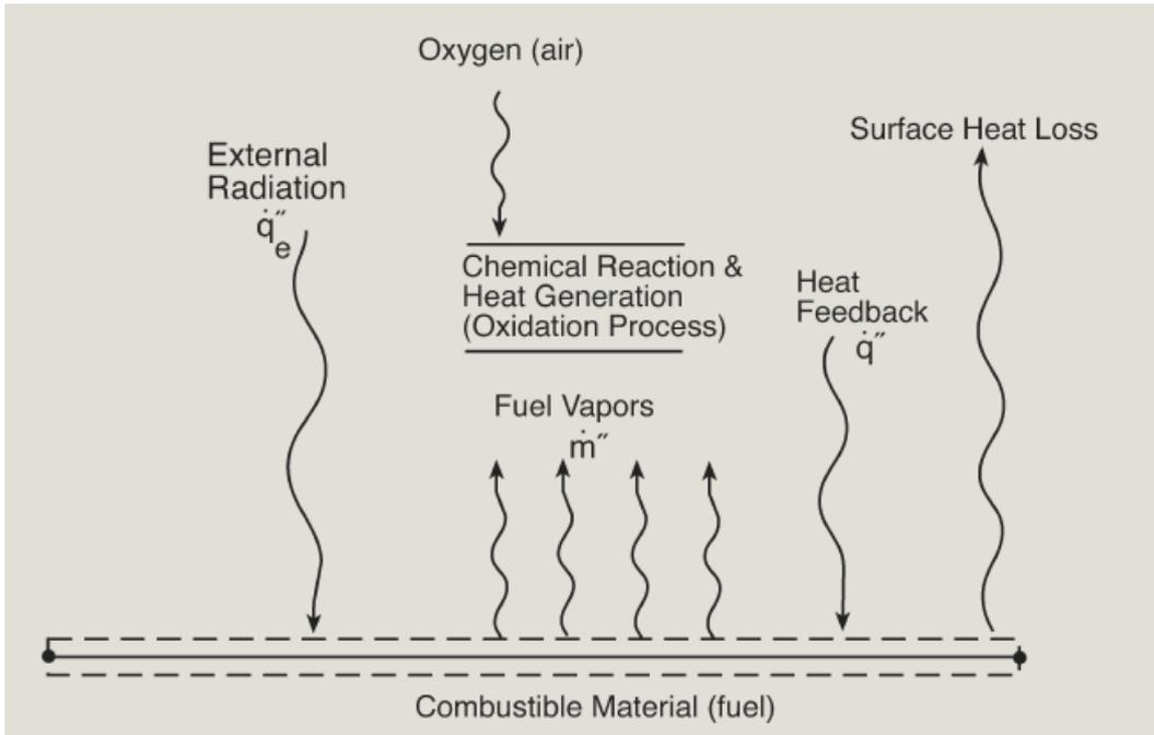
**Figure 4:** Physical process of a fire
