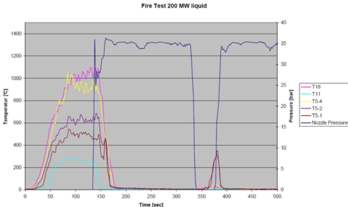
**Figure 3:** Temperature measurements - 200 MW liquid fire test
