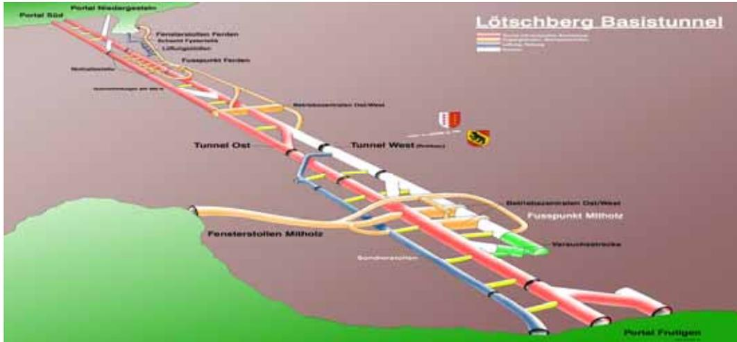
**Figure 1:** Sketch of the Lötschberg Base Tunnel
