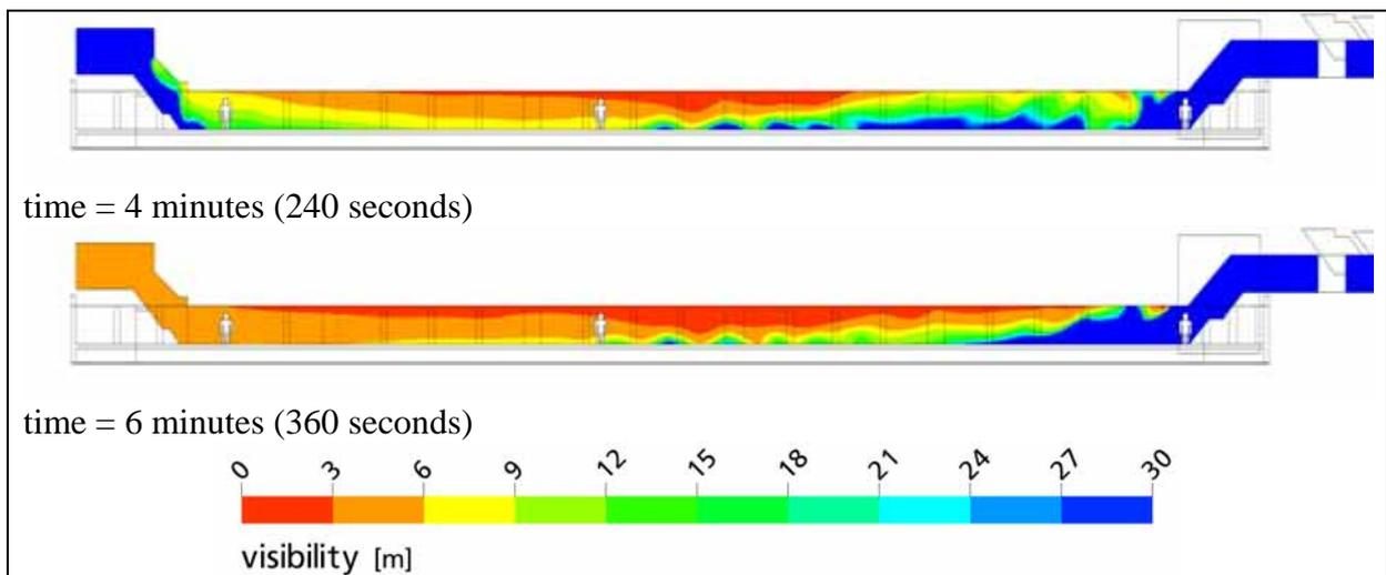
**Figure 9:** Visibility plots, centre of station, push pull ventilation
