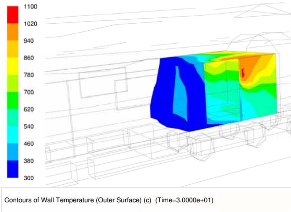
Figure 7: Inside train wall temperature above ignition temperature (set to be 300°C)
