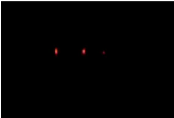
This image shows just 3 beacons, so the vision distance is 10 m. This image shows (by way of example) the situation a few minutes after ignition of a fire.
