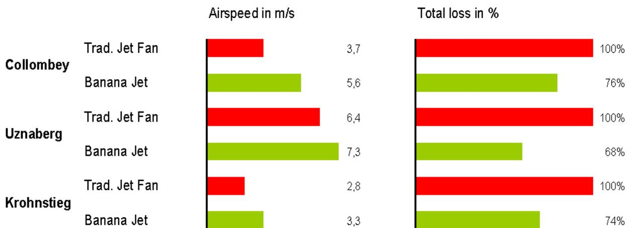
Figure 4: Comparison of measured airspeed in the tunnel
