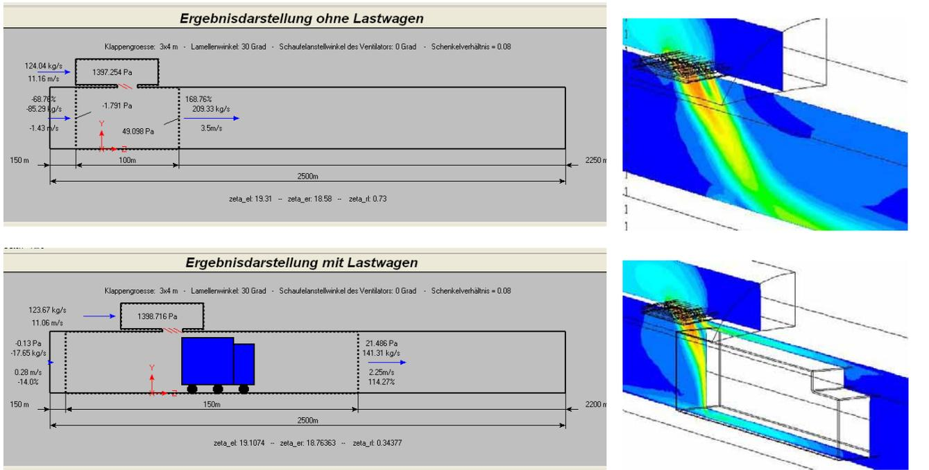
Figure 5: Comparison of results with and without a truck in the traffic room.
