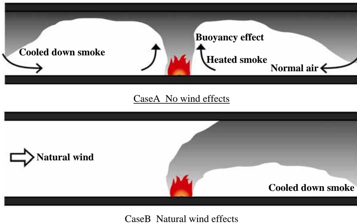
**Figure 2-1:** Basic description of smoke behaviour
