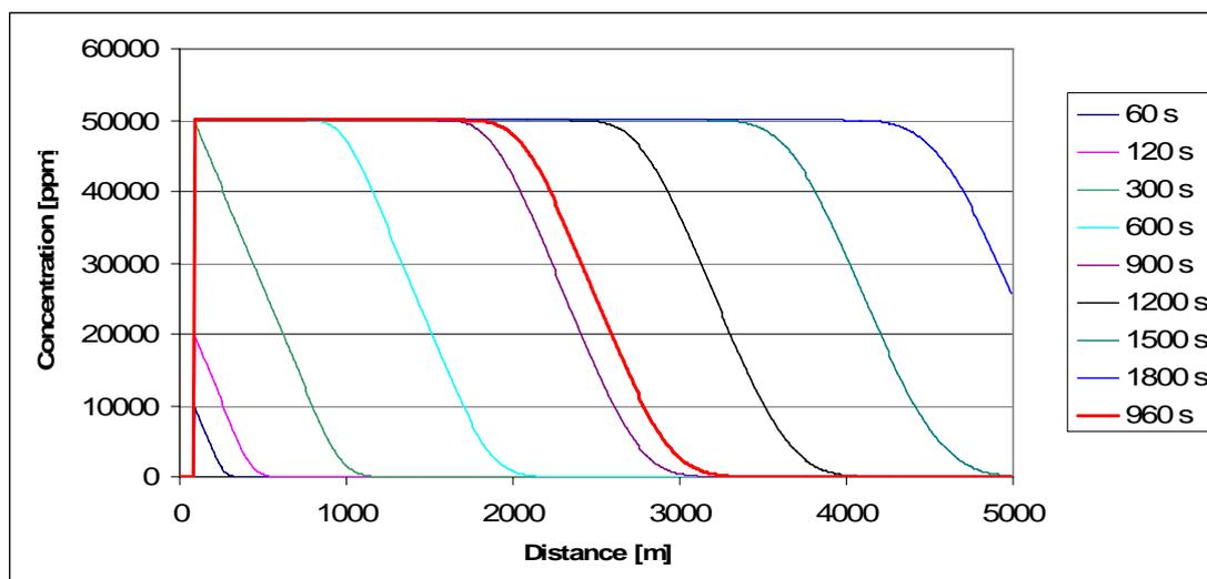
**Figure 4:** Dispersion of chloride in the tunnel after a leak (50mm) of a vessel (ventilation speed 3 m/s).
