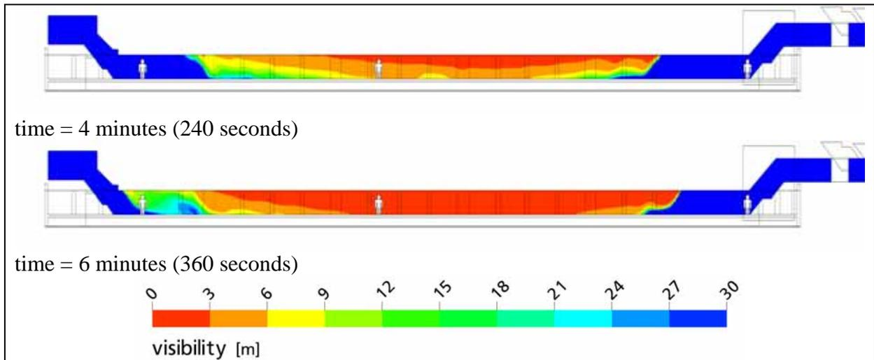
**Figure 8:** Visibility plots, centre of station, all-exhaust ventilation
