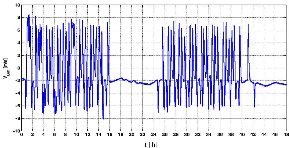
**Figure 2:** Measured longitudinal air speed during a period of normal train operation in the LBT. During operation off hours (in the night) the residual longitudinal airflow is based on the thermodynamic buoyancy effect of the sloped tunnel and the meteorological boundary condition at the tunnel portals.
