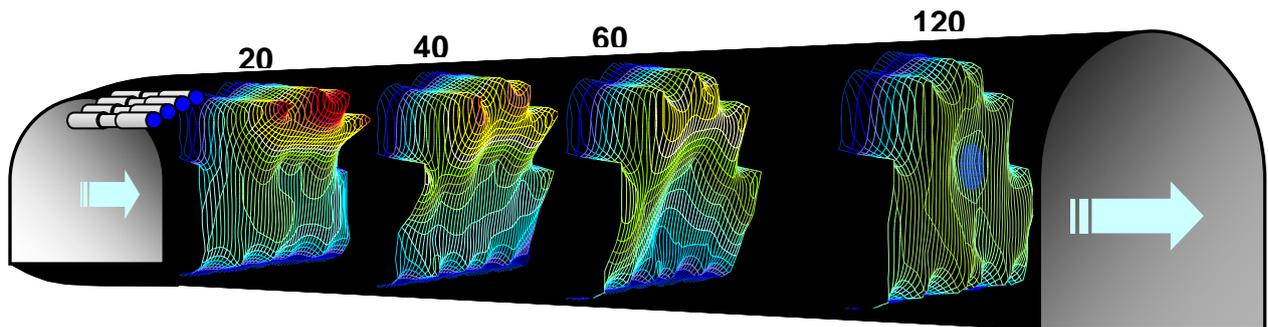
**Figure 7: Air speed profile across the tunnel cross section of Uznaberg West tunnel Traditional Jet Fan**
