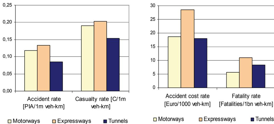
**Figure 1:** Relative accident rates for tunnels versus motor- and expressways (1999-2007)
