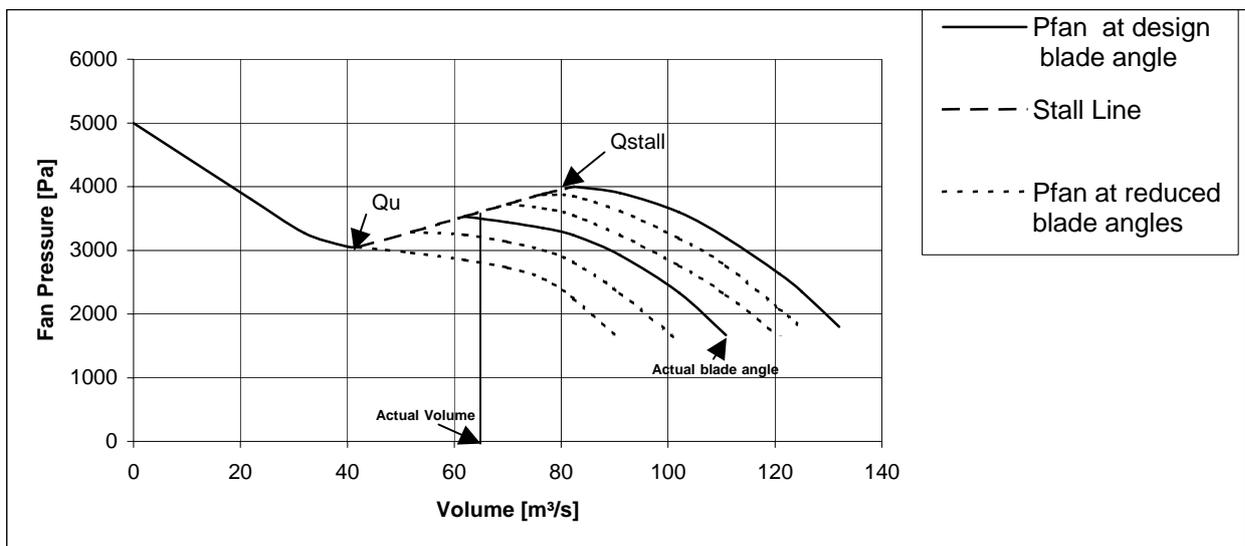
**Figure 2: Fan curve variable pitch fan**
