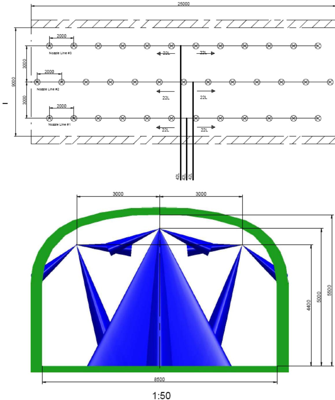
**Figure 1:** Plan view of one section and cross section: the Spray Nozzles and Nozzle Lines in the test tunnel
