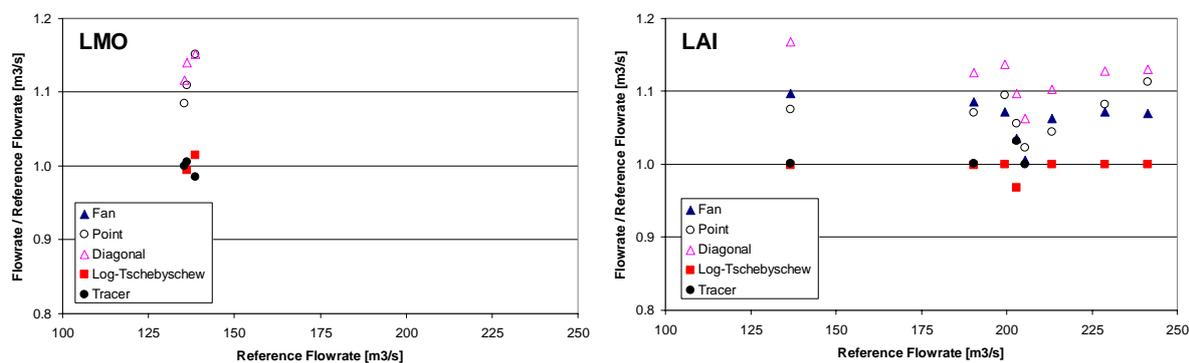
**Figure 4:** Comparison of the different measuring techniques tested in the Gotthard road tunnel, measuring station in the tunnel (left) and close to the ventilation station Airolo (right).
