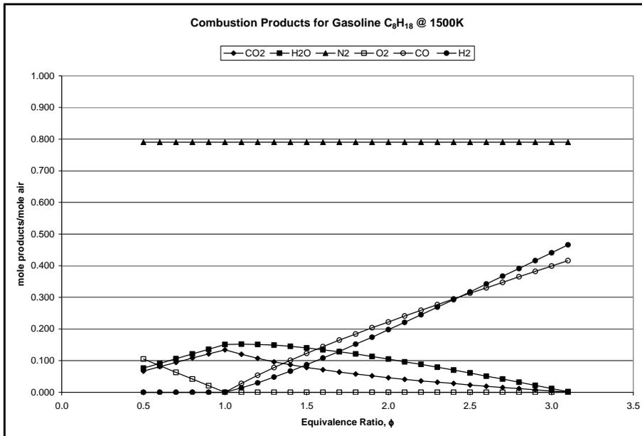
Figure 3: Combustion product for gasoline as a function of  $\phi$  at T=1500K
