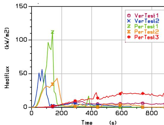
**Figure 9:** Mean heat flux in the ‘wet’ part of the test tank
