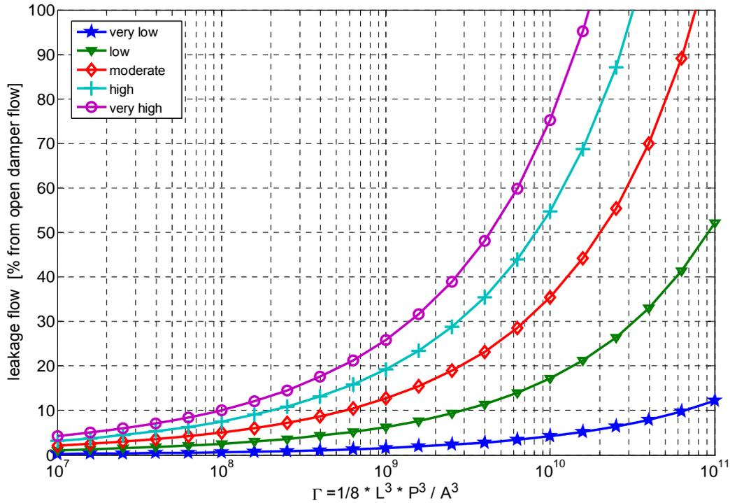
**Figure 5:** Graph to estimate the expected leakage flow
