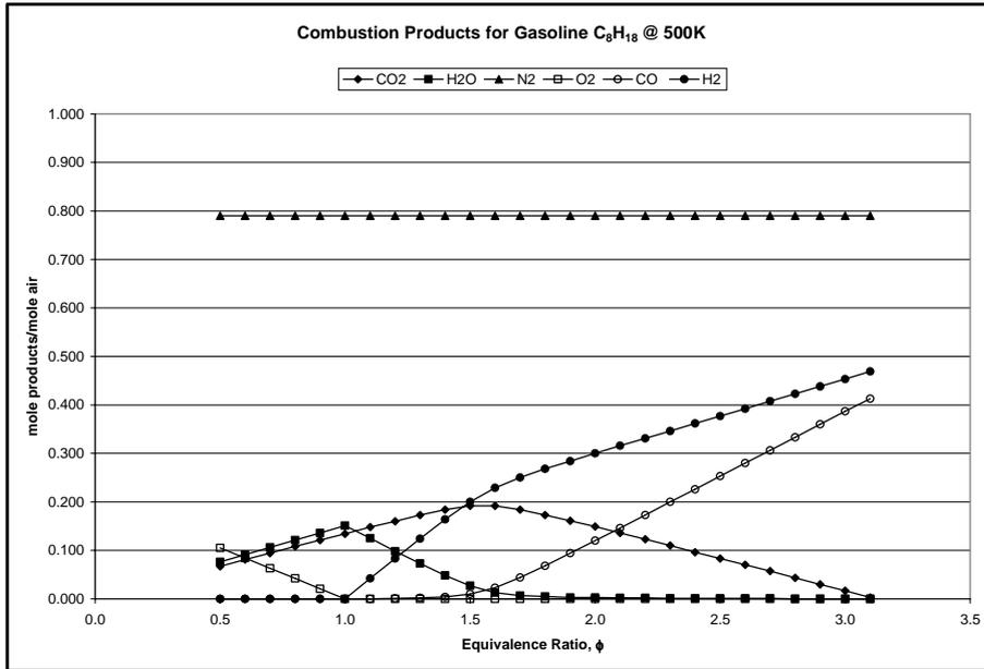
Figure 2: Combustion product for gasoline as a function of  $\phi$  at T=500K
