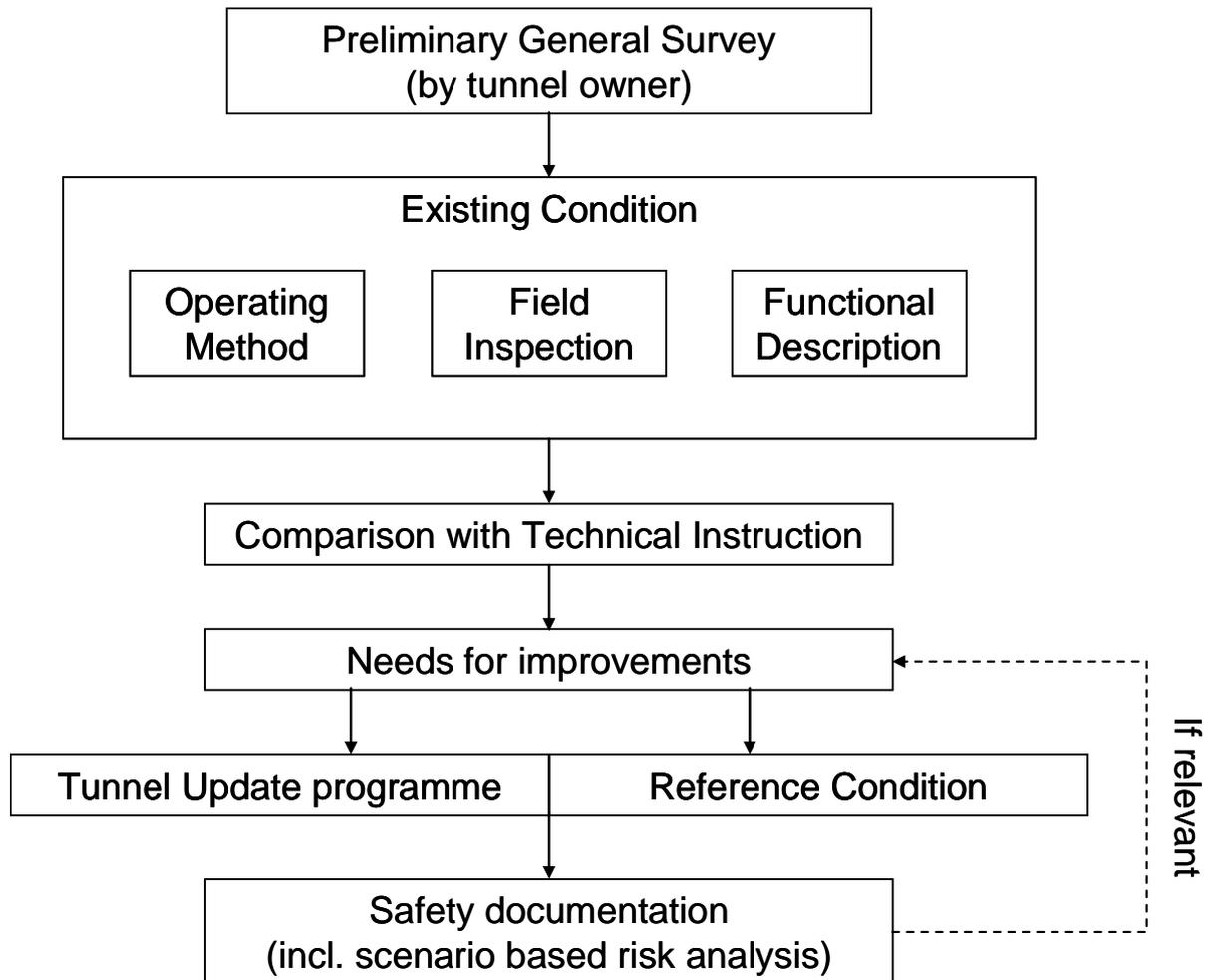
**Figure 1:** Specific process for tunnels in operation, so as to define an acceptable level of safety. Derived from [2]
