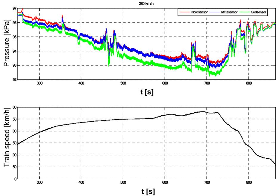
**Figure 6:** Pressure fluctuation on a passenger train (ICE) at different position on the train while passing the Lötschberg Base Tunnel. On the left side: Pressure sensors installed on the window of the train. On the right side: Measured pressure fluctuation on the train (outside) while passing the tunnel and the correspondent speed profile of the passenger train.
