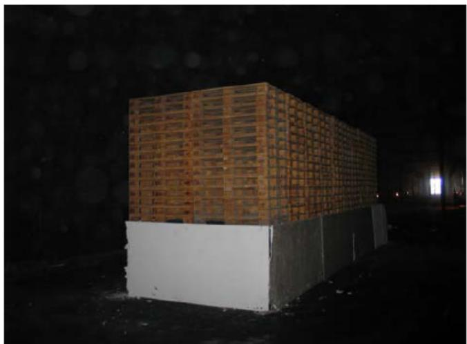
**Figure 15+16:** 2 x 14 x 9 pallets on a 1,1 m high stand
