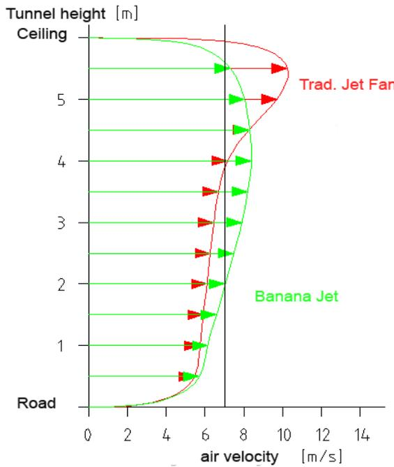
**Figure 1: Average flow rate in a tunnel (Uznaberg West)**
