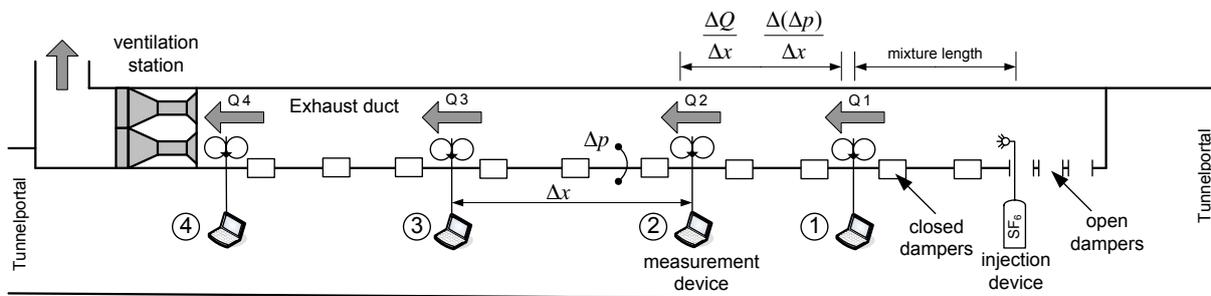
**Figure 2:** Sketch of the tracer gas measurement set up
