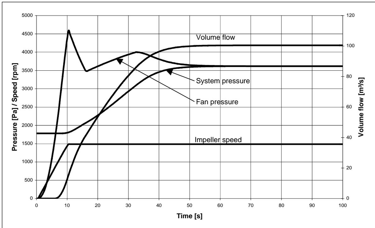
Figure 8: Start-up second fan with variable pitch fan
