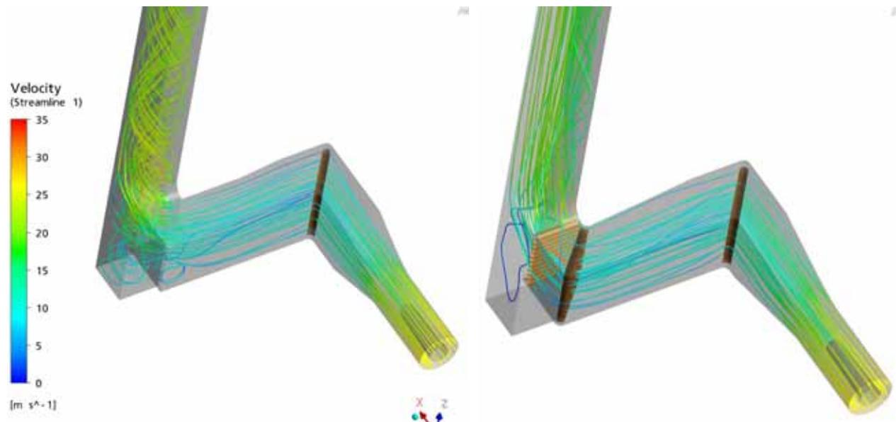
**Fig. 3.:** Streamlines of current design (left) and after (right) integrating the guiding vanes. The colours of the streamlines correspond to the velocity
