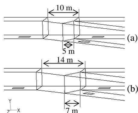
**Figure 4:** The junction zone of the tunnel, for the width of the lateral branch of (a) 5 m, (b) 7 m
