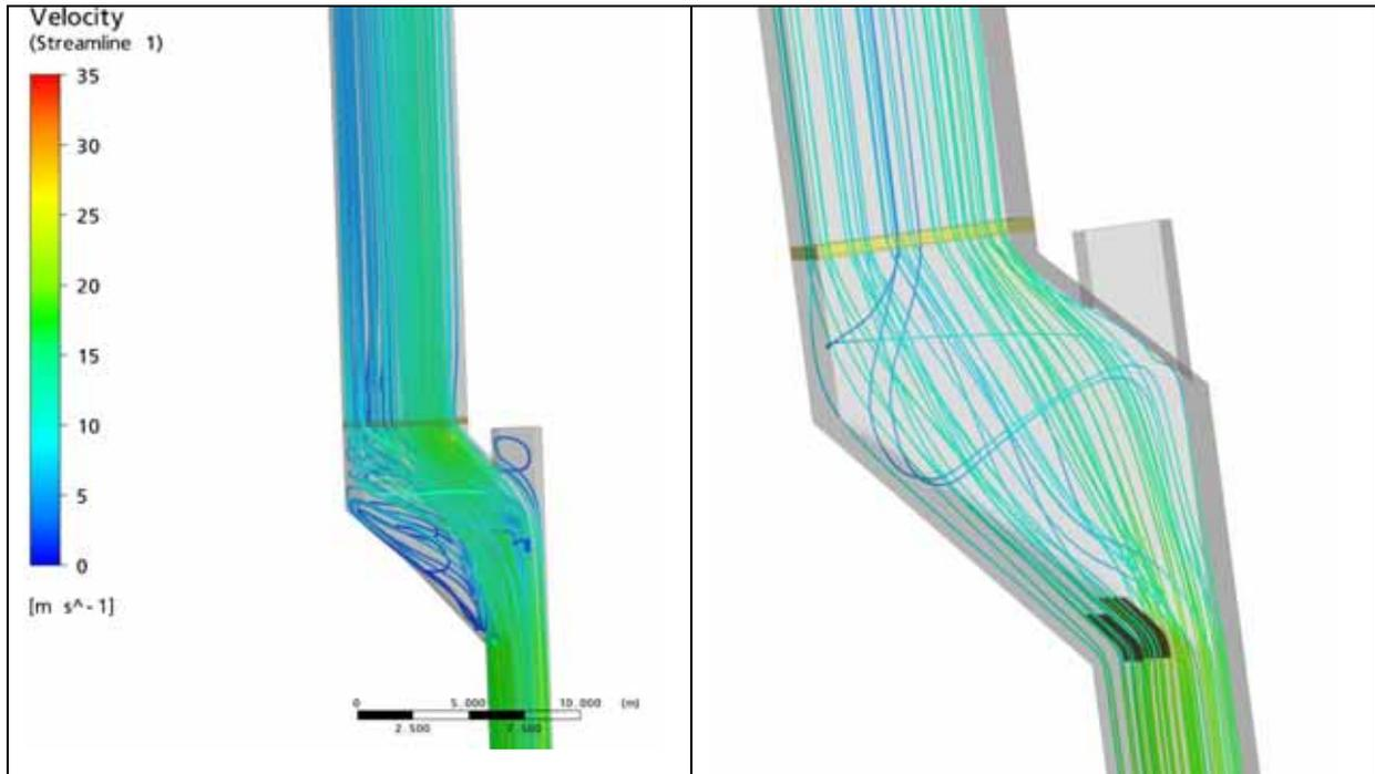
**Fig. 4.:** Streamlines of current design (left) and after (right) integrating the guiding vanes in the funnel branching. The large detachment area is minimized by applying two guiding vanes.
