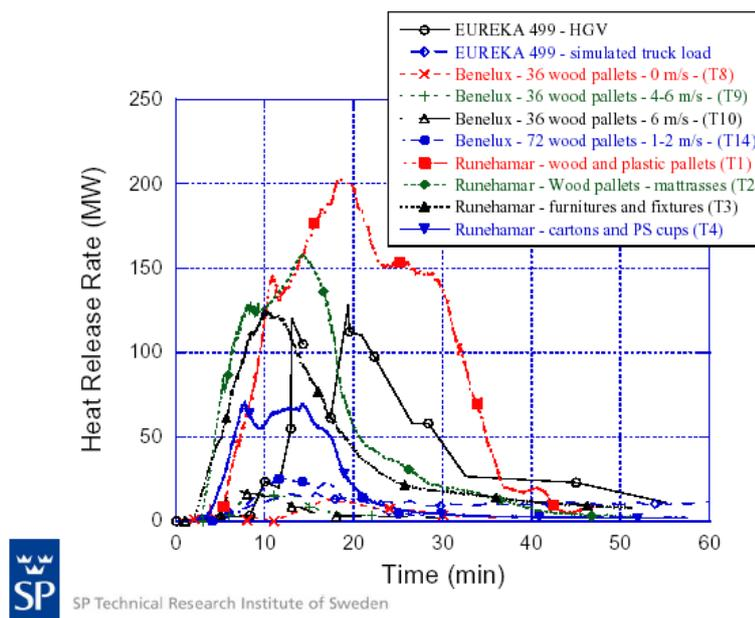
**Figure 1:** Summary of test data on fire growth rates (note importance at first 5 minutes).
