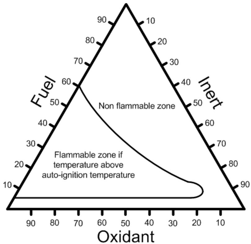
**Figure 5:** Generic vapor phase flammability diagram
