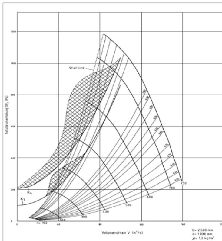
**Figure 6:** Fan performance chart with systems resistance characteristics  $K_1$  and  $K_4$
