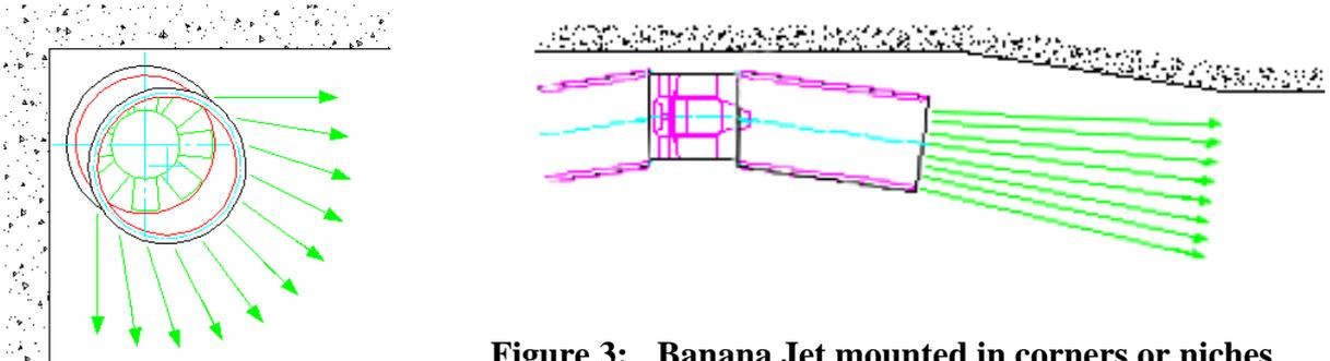
Figure 3: Banana Jet mounted in corners or niches
