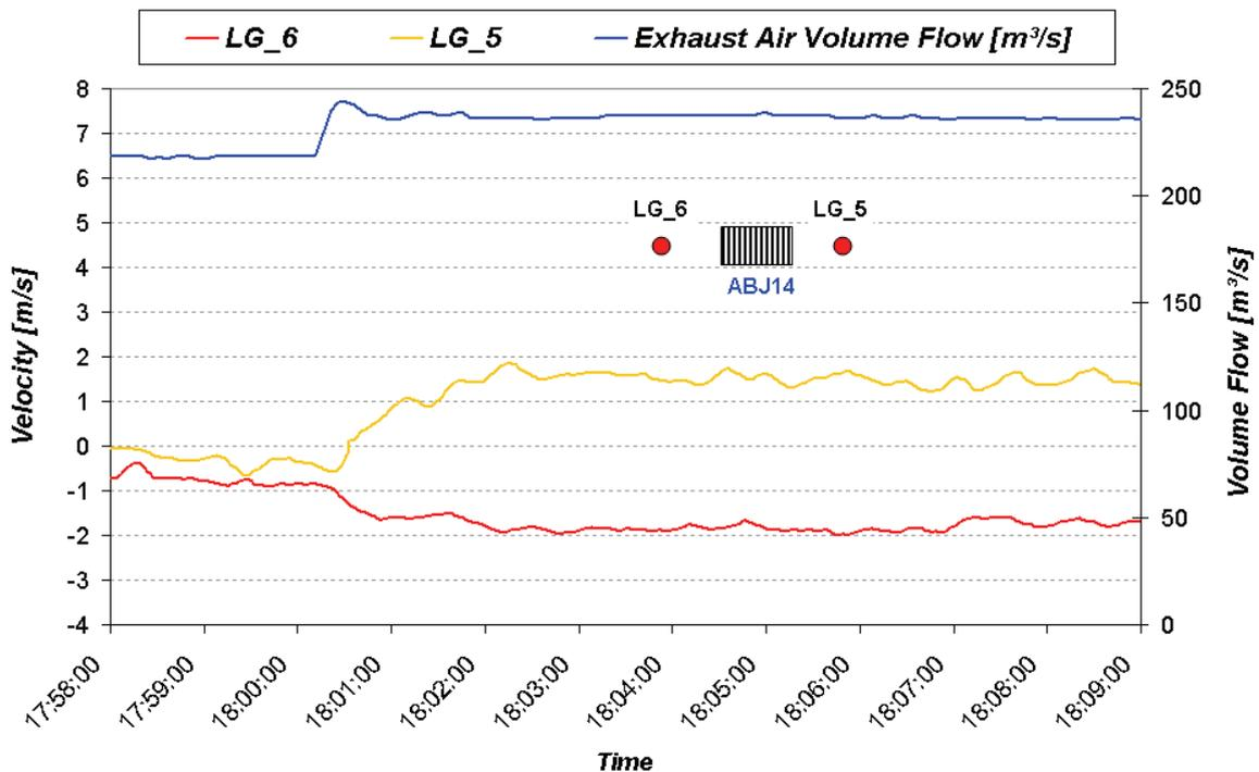
**Figure 7:** Air velocity vs. time during a fire test, bidirectional traffic mode
