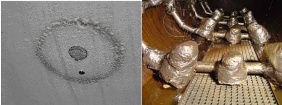
**Figure 5:** Mounting of the heat flux sensors in the tank wall - external and internal views
