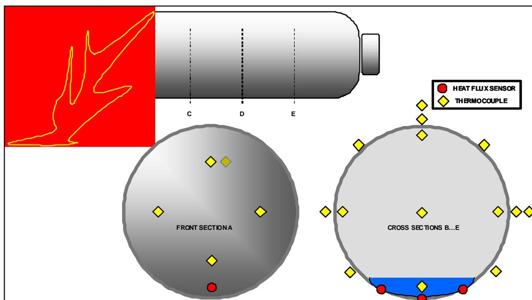
**Figure 6:** Positions of the heat flux meters and thermocouples
