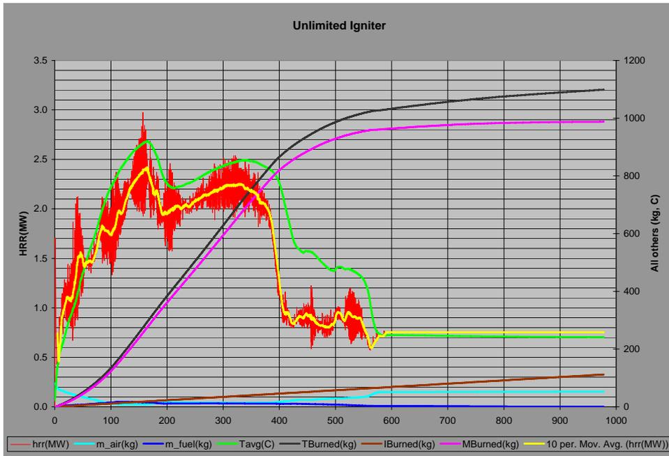
Figure 6: FHRR predictions in a train car in a tunnel
