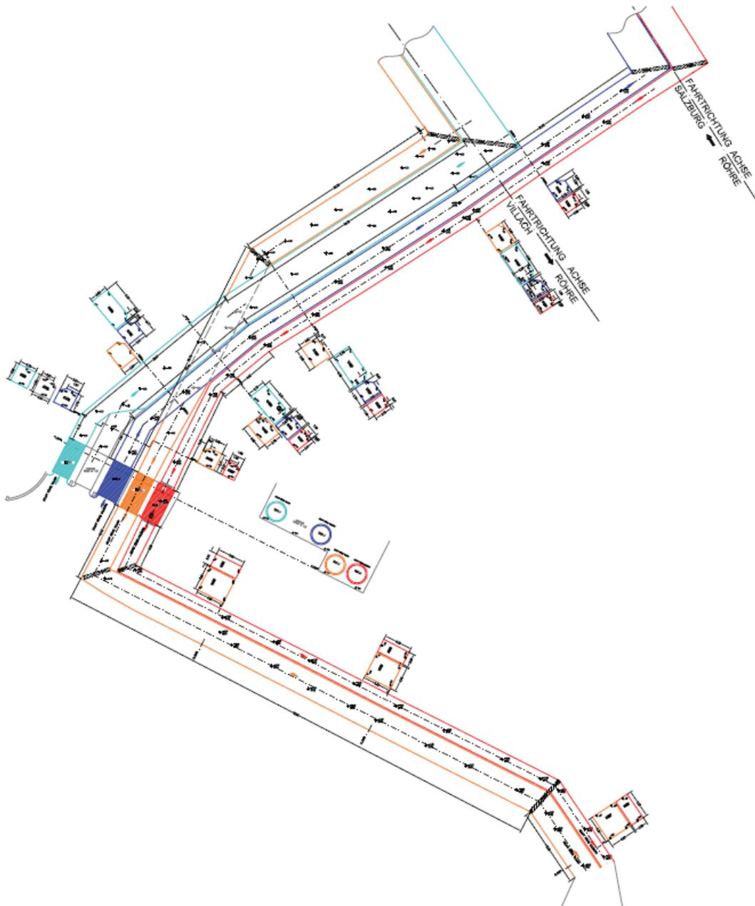
**Figure 5:** Plan view of the fresh-air and exhaust-air ducts of the Tauern tunnel ventilation section south, ventilation building south
