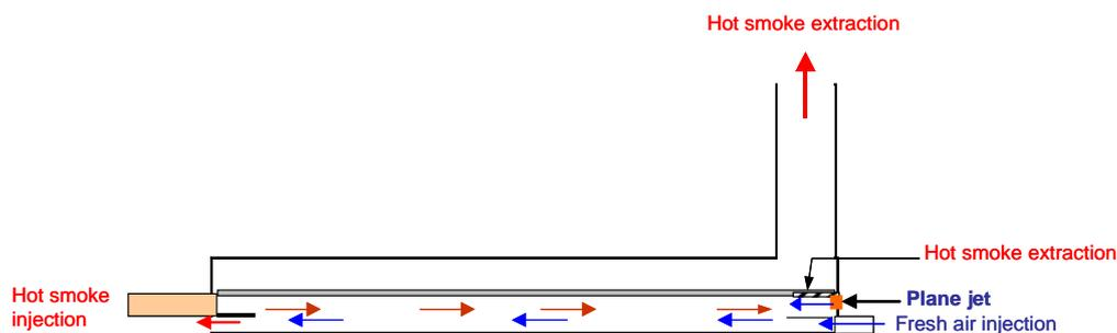
**Figure 4 :** Experimental set-up for studying interaction between fans and the smoke layer.
