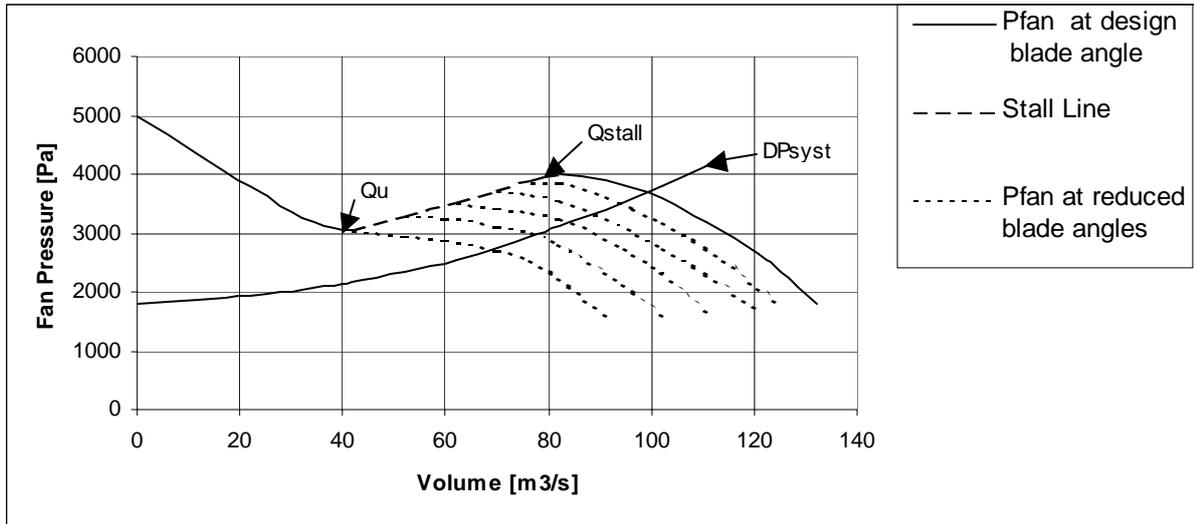
Figure 7: System resistance line and variable pitch fan curve
