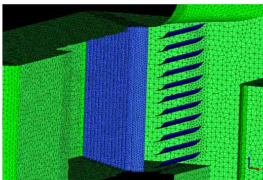
ICEM grid with the new adapted Guiding vanes (blue) in the corner 2 and at the access to the funnel.
