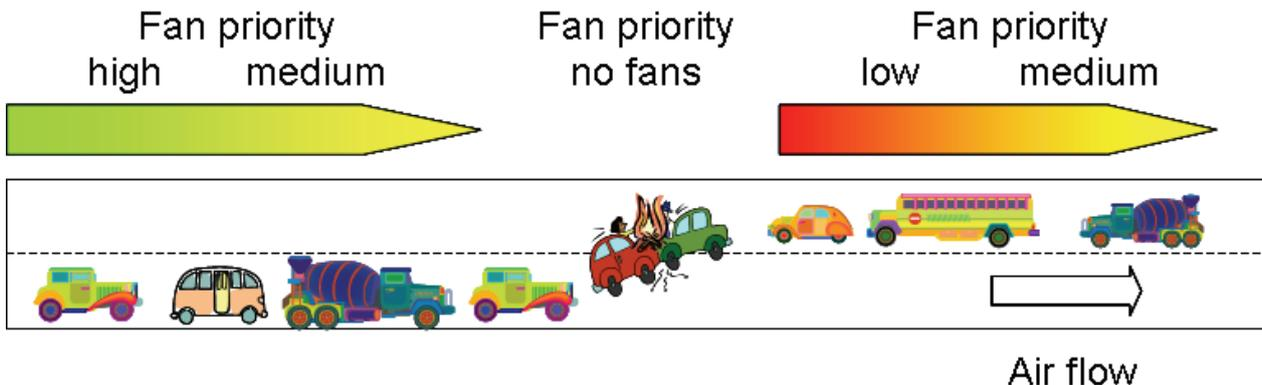
**Figure 2:** Ventilation philosophy for longitudinally ventilated tunnels with bidirectional traffic
