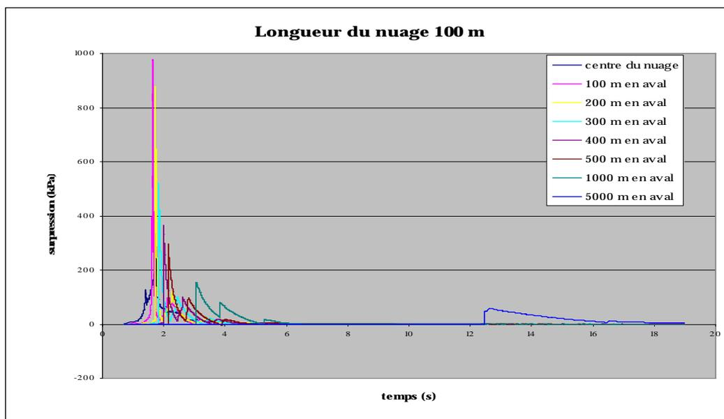
**Figure 2:** The blast effects after ignition of a cloud with a length of 100 meter
