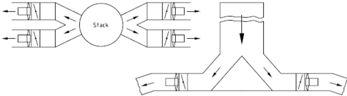
**Figure 5:** Fan installation in parallel operation
