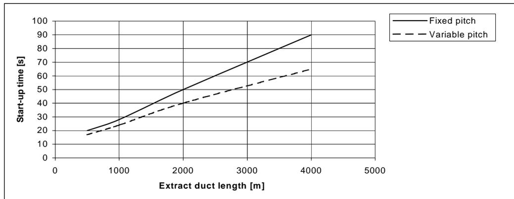
**Figure 9: Influence duct length on start-up time**
