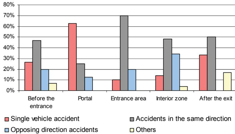
**Figure 4:** Types of accidents in tunnels with bi-directional traffic by point of origin of the accident, in percent (1999-2007)
