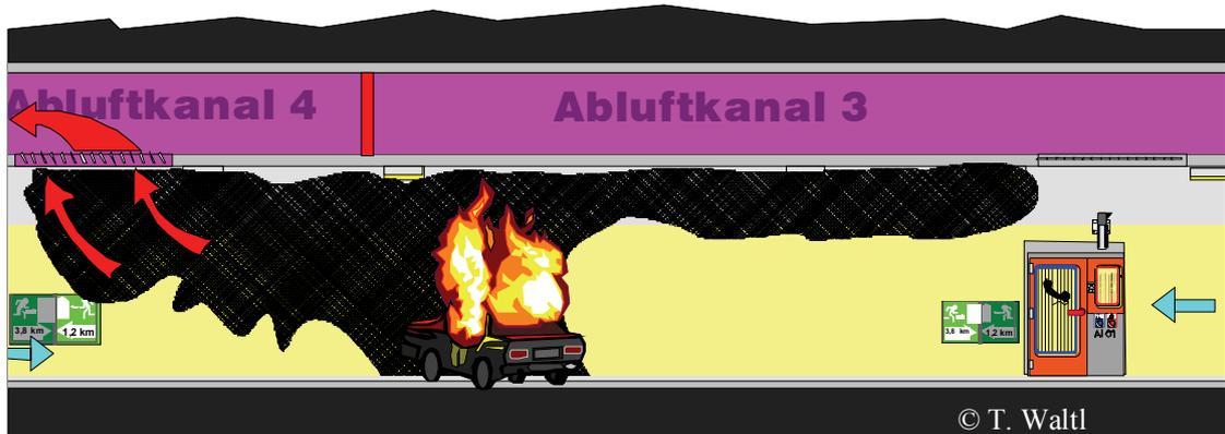
**Figure 3:** Ventilation philosophy for transverse ventilated tunnels
