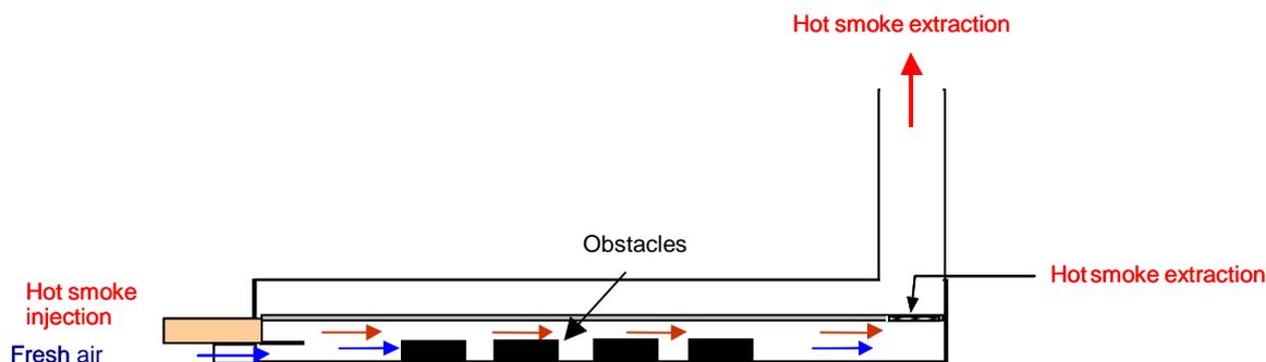
**Figure 3** : Experimental set-up for congested vehicles disturbance effect.
