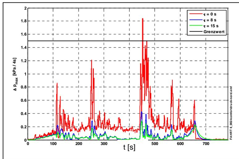
**Figure 7:** Measured maximum pressure fluctuation within time periods of 4 seconds in the train during its journey through the tunnel (see figure 6). These calculated pressure fluctuations inside the passenger train quote for different sealing factors  $\tau$  of the train. The dashed horizontal line indicates the comfort criteria of 1.5 kPa/4s. The pressure profiles prove that the comfort criterion is fulfilled only with a sealed passenger train ( $\tau > 0$ ).
