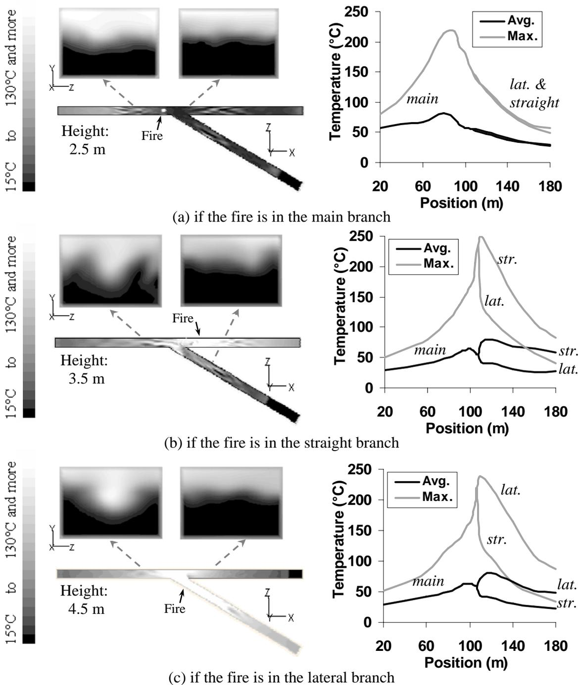
**Figure 2:** The temperature in the air: 1) the field, 2) the maximum and the average values along the tunnel
