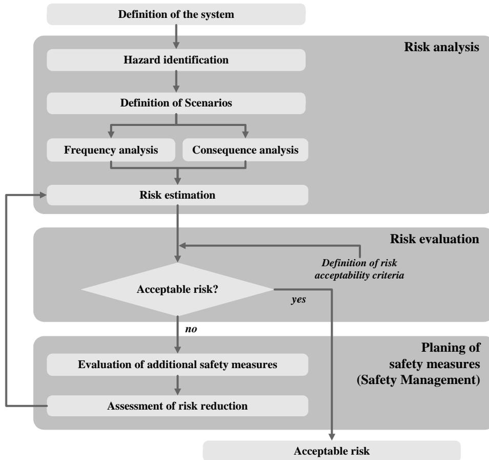
**Figure 1:** Procedure for a system-based risk assessment
