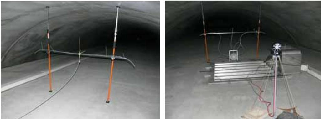
**Figure 5:** Measuring techniques in the Branisko tunnel. Left: SF<sub>6</sub> injection; right: SF<sub>6</sub> suction and velocity measurement. The damper shown in the right picture was sealed by a steel plate.
