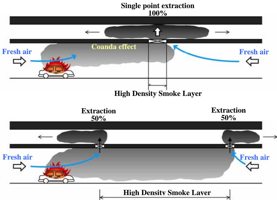
Figure 2-5: Difference of smoke layer between single and multi extraction port
