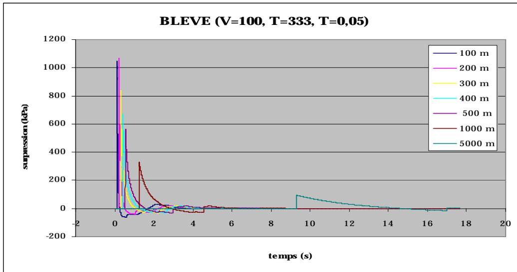
**Figure 3:** Possible blast after a BLEVE of a vessel of 100m<sup>3</sup>
