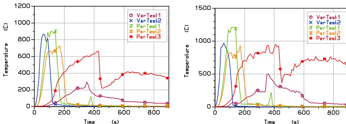
**Figure 7:** Mean temperature (left) and maximum temperature (right) of the air around the test tank
