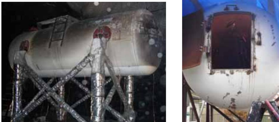
**Figure 4:** The test tank in the tunnel and the access door that was cut in the end wall.
