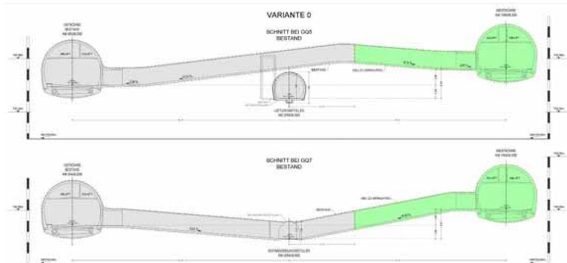
**Figure 2:** Position of the existing cross-vents (grey) and the continuation according to the general project from 1979
