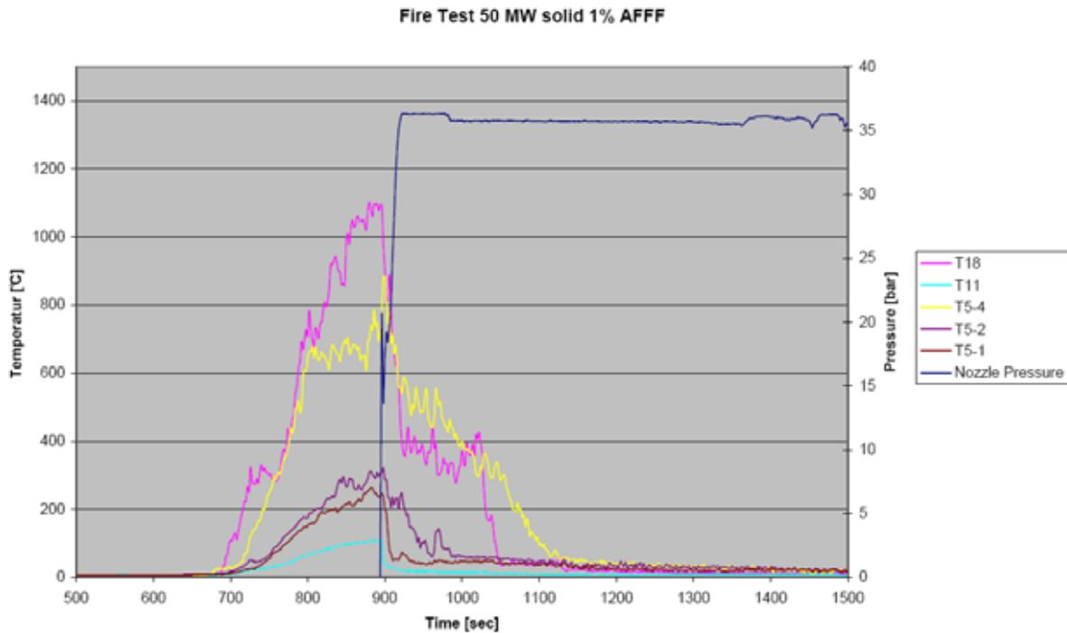
**Figure 2:** Temperature measurements - 50 MW solid fire test
