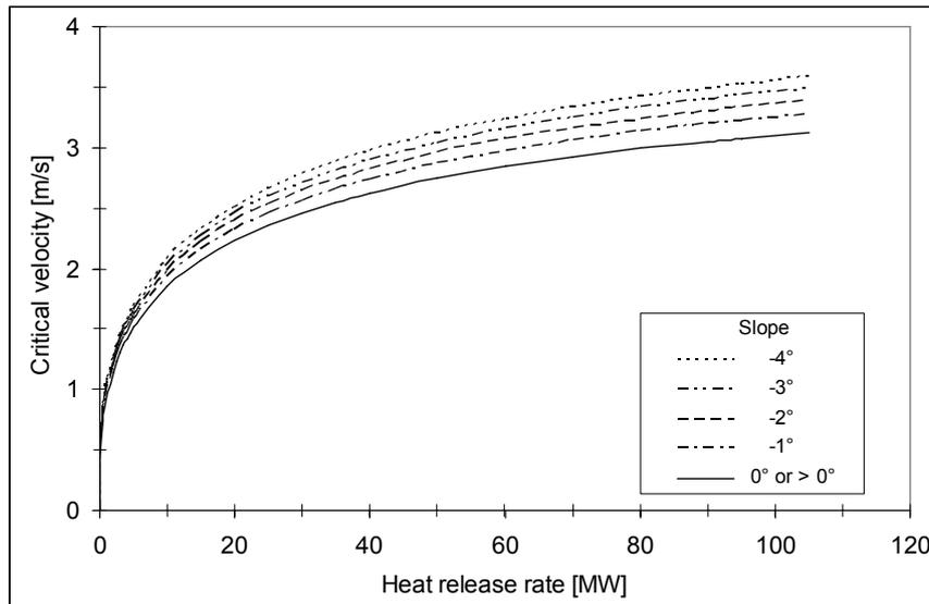
**Figure 1:** Critical velocity for a typical 60 m<sup>2</sup> tunnel with slopes between -4 % and 0%.
