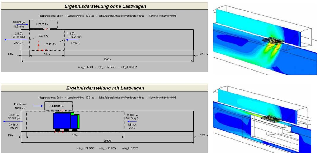
Figure 6: Comparison of results with and without a truck in the traffic room.
