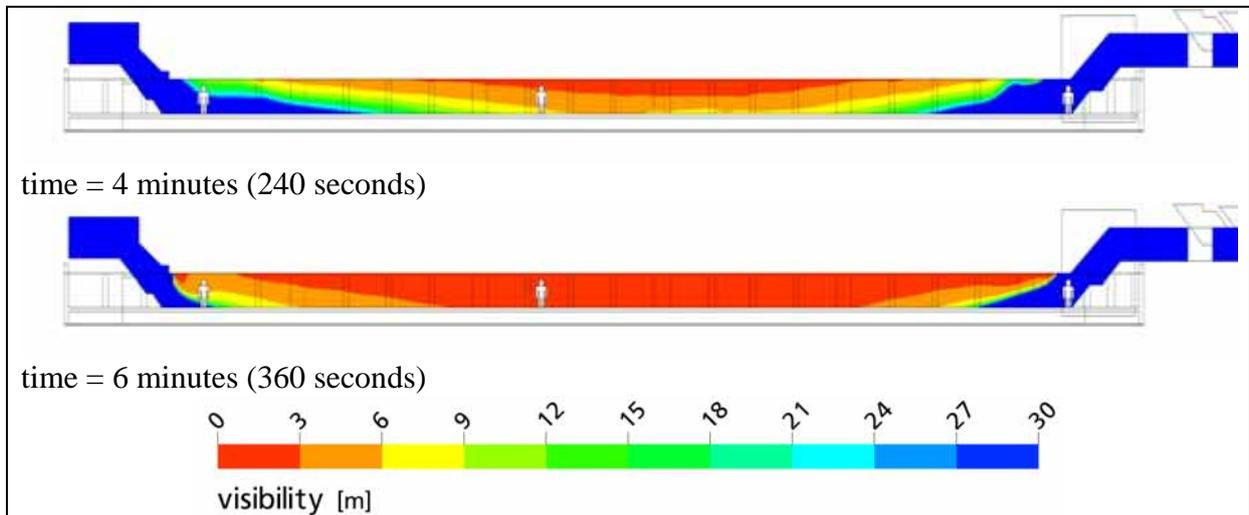
**Figure 7:** Visibility plots, centre of station, natural ventilation
