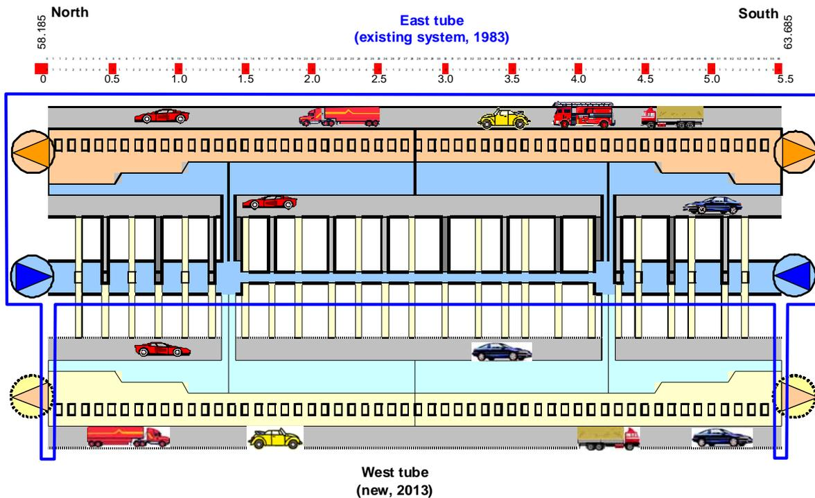
**Figure 1:** Ventilation concept as anticipated in the initial project (existing system in rectangle)
