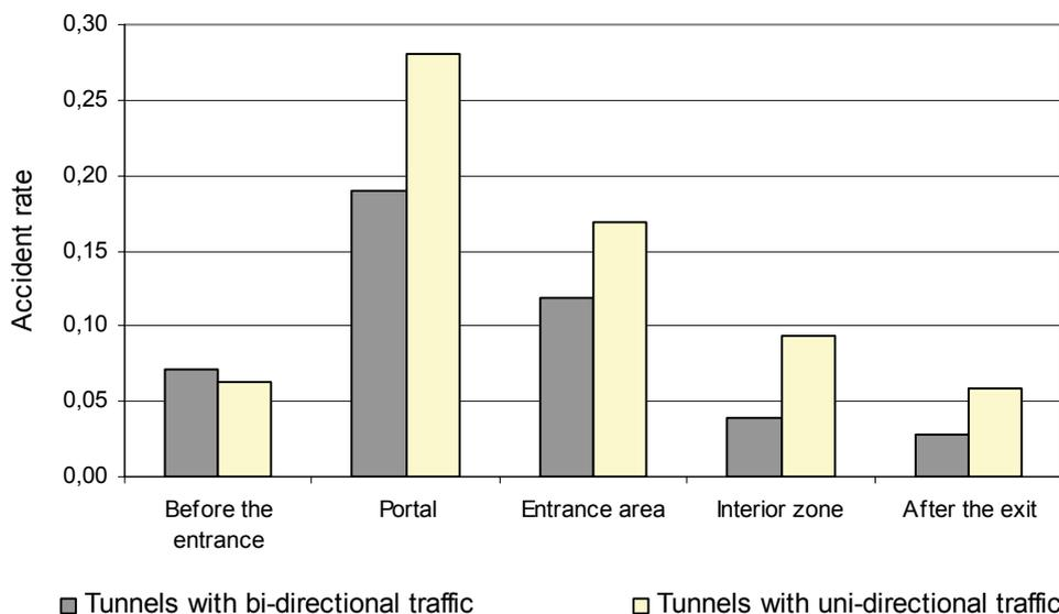
**Figure 3:** Personal injury accident rate [PIA/1 million vehicle-kilometres] in tunnels with bi-directional traffic and unidirectional traffic by point of origin of the accident (1999-2007)
