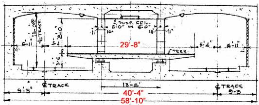
**Figure 4:** Cross section of station platform
