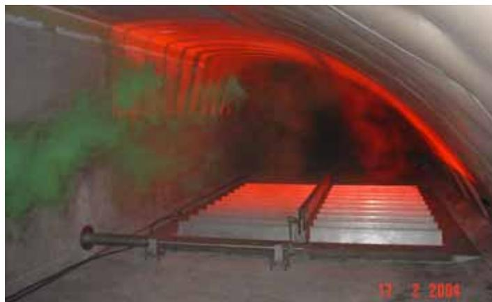
**Figure 1:** Exhaust air flap in the verification test
