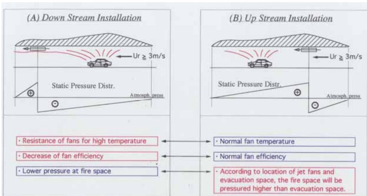
**Figure 2-3:** Relation ship between Static pressure distribution and location of Jet fans
