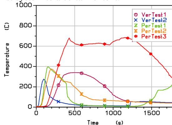
**Figure 8:** Maximum temperature of the wall of the test tank. Note: the increase in temperature in PerTest 1 is caused by the after-burning of the fuel and is not part of the official test.
