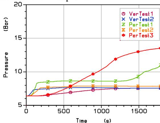
**Figure 10:** Pressure of LPG in the reference tank calculated from measured heat fluxes and wall temperatures of the test tank.
