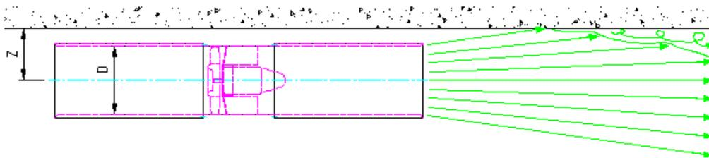
**Figure 2: Impulse and friction losses behind a traditional jet fan**
