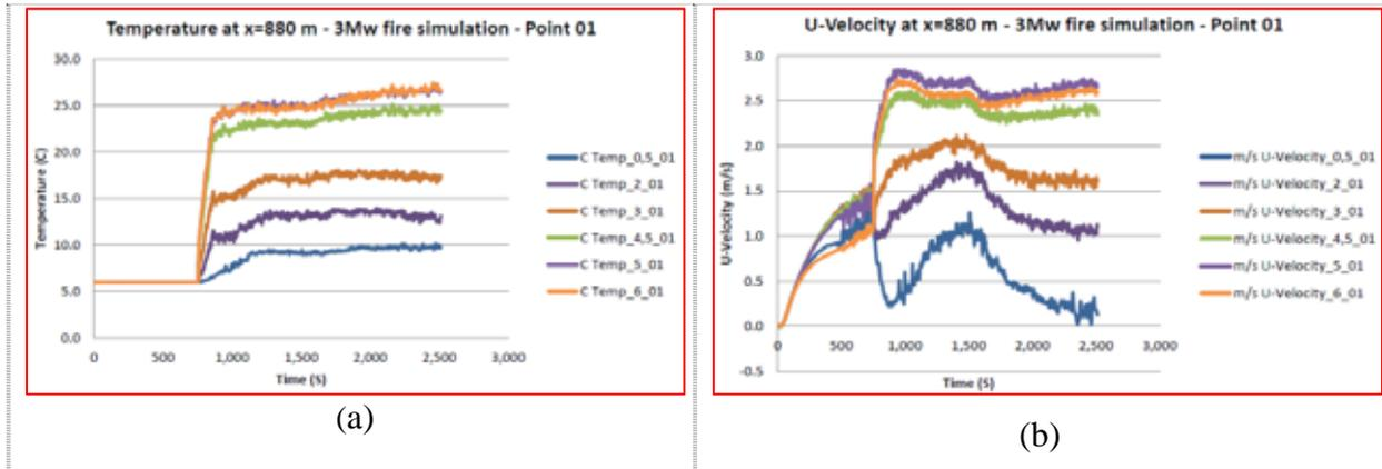
**Fig. 5:** Temperature (a), U-velocity (b) at tunnel cross section 01, 3MW case
