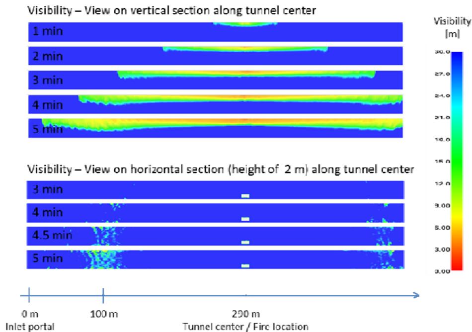
**Figure 5:** CFD results for fire situation with congested traffic and natural ventilation
