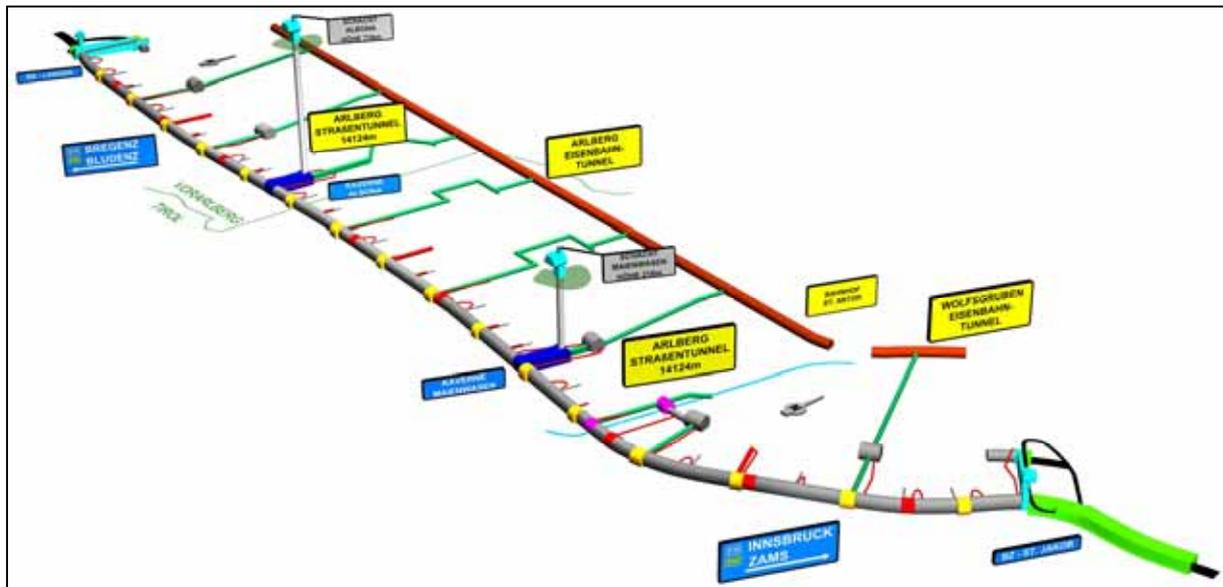
**Figure 4:** Sketch of the egress ways of the Arlberg tunnel (AISFINAG).
