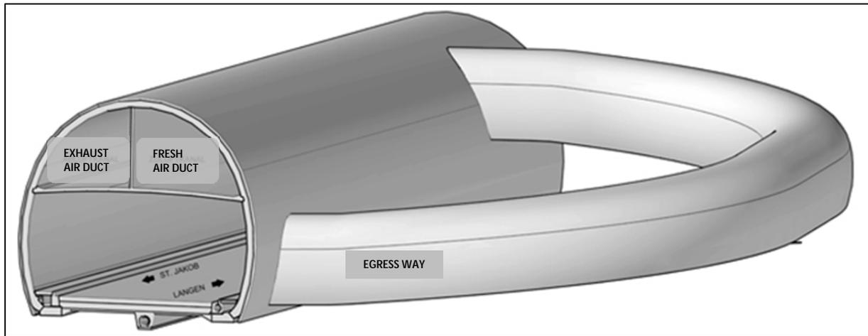
**Figure 8:** Scheme of the new egress way (ASFINAG).
