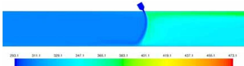
**Figure 12:** Temperature range in cross section  $e=5$  cm,  $U=10$  m/s (K)
