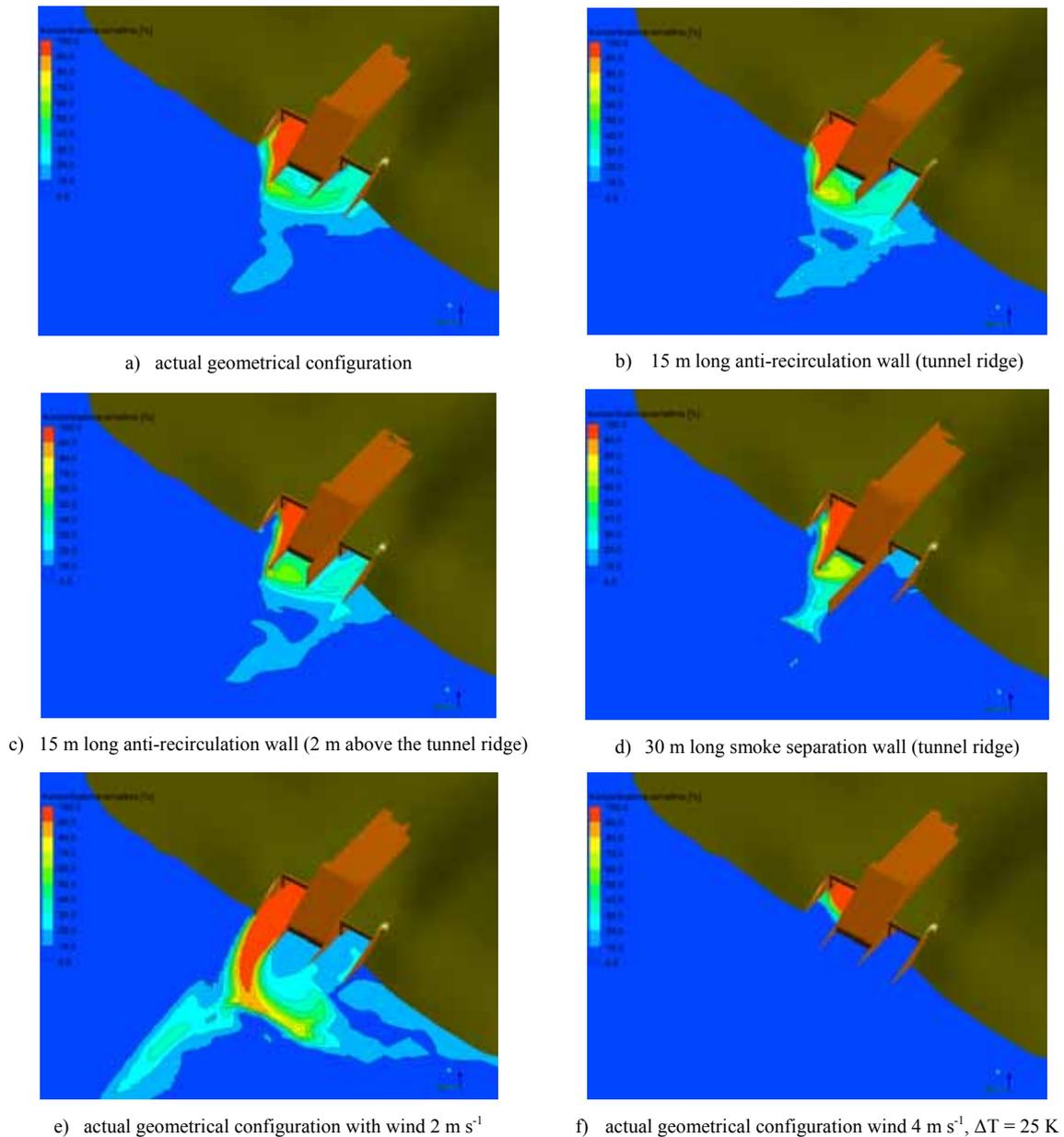
**Figure 5:** Recirculation level at 1 m above the tunnel floor level
