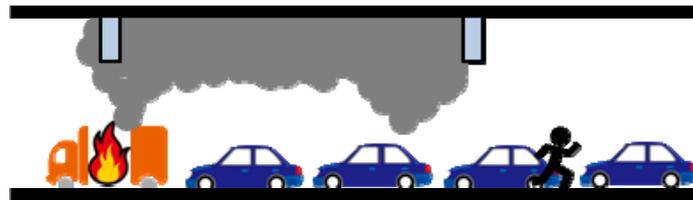
**Figure 1:** Schematic diagram of the effect of a smoke barrier in the case of fire.
