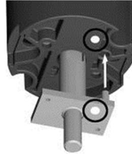
Recalibration with checking rod
