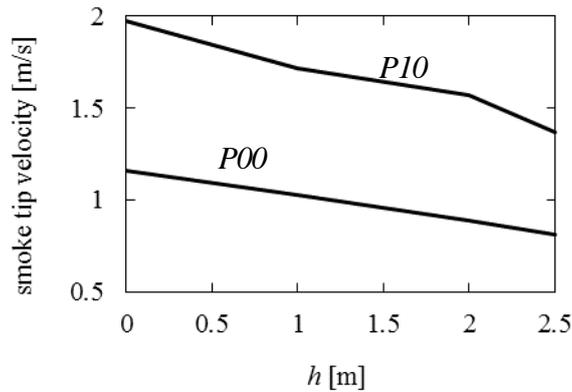
**Figure 6:** Influence of smoke tip velocity by smoke barrier in the case of  $s = 0\%$
