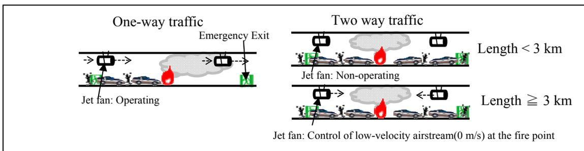
**Figure 6:** Principle of smoke control of longitudinal ventilation systems (Inter-city tunnel)
