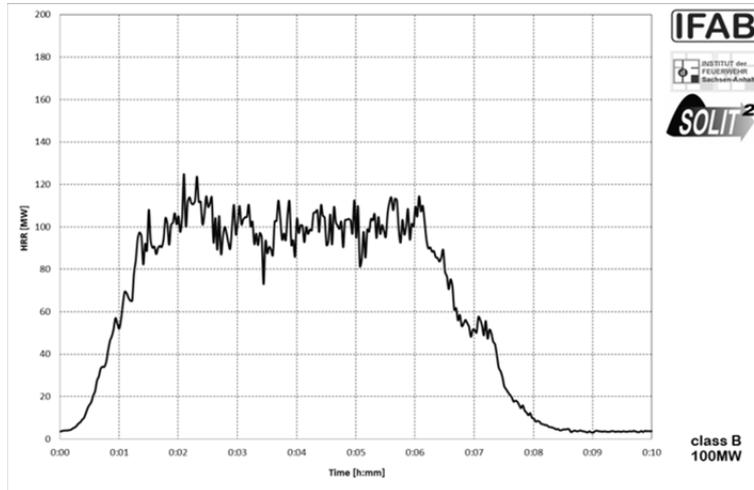
**Figure 3:** Heat release rate for a 100 MW class B fire test
