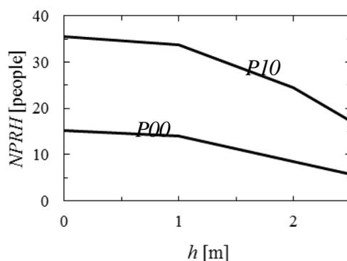
**Figure 7:** Change in  $NPRH$  with smoke barrier height in the case of  $s = 4\%$
