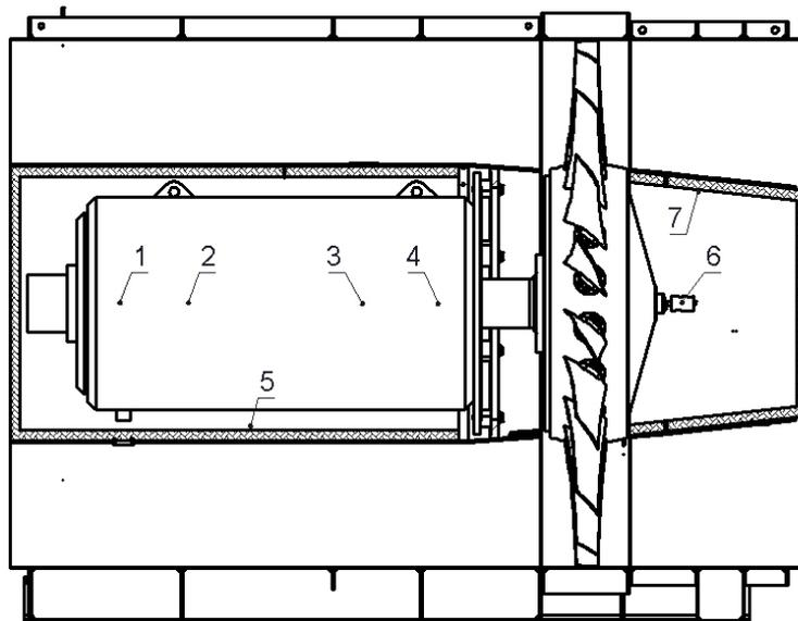
**Figure 4:** Thermocouples arrangement
