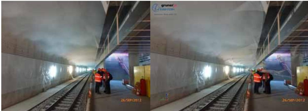
**Figure 4:** Actual and simulated smoke density during test 2 in the station
