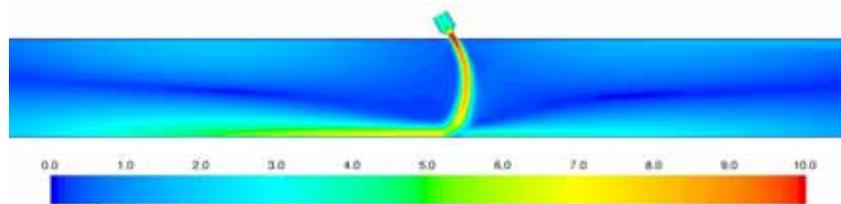
**Figure 13:** Velocity profile in cross section  $e=10$  cm,  $U=10$  m/s
