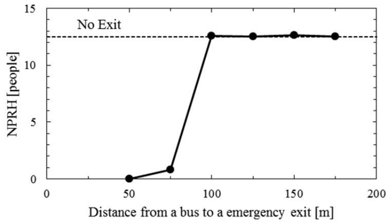
**Figure 10:** Effectiveness of the emergency exit,  $\Delta 0\text{Pa}$
