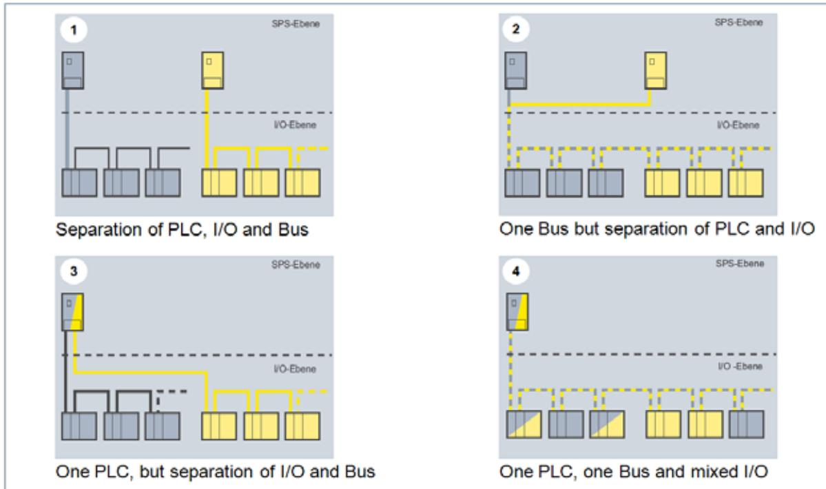
**Figure 2:** Fail-safe design variations (yellow components are fail-safe modules)
