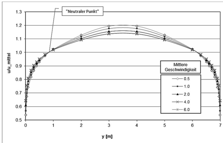
**Figure 2:** Pipe flow velocity profile
