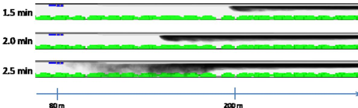
**Figure 2:** Destruction of stratified smoke layer by activation of jet fans (in this example the jet fans shown above are started at 2 minutes according to scenario timeline)
