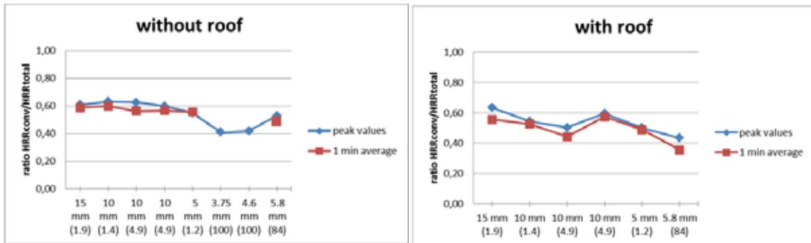
**Figure 1:** The measured ratio of convective HRR ( $HRR_{conv}$ ) and total HRR ( $HRR_{total}$ ) for different water densities (mm) and pressures (bar), both without and with roof above the fuel mock-up.
