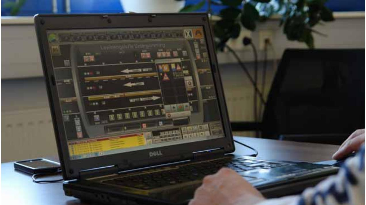
**Figure 8:** Micro control console as notebook control console with tunnel remote control
