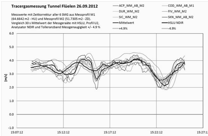
**Figure 4:** Tunnel Flüelen, measured data and tracer gas values
