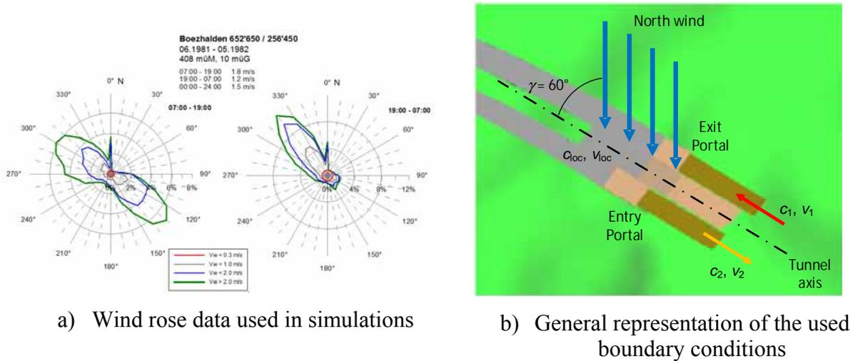
**Figure 4:** Boundary conditions used in numerical simulations
