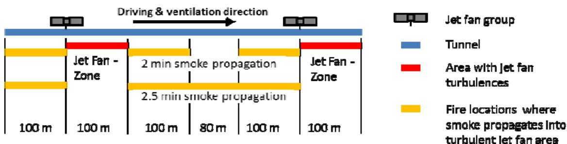
**Figure 3:** Illustration of fire locations where activation of jet fans would result in destratified smoke propagation for fan installation in the tunnel
