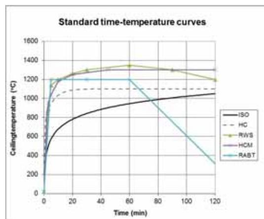
**Figure 2:** The most common standardized time-temperature curves for road tunnel applications.
