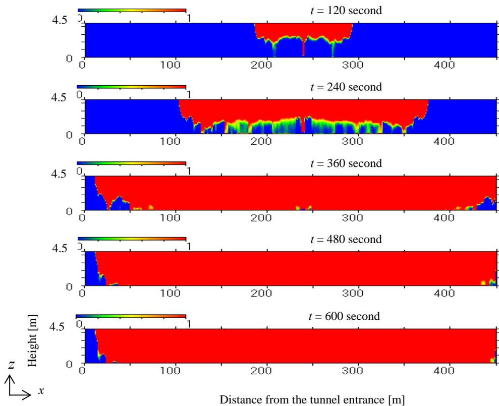
**Figure 9:** Smoke density distribution in the x-z plane across the tunnel model
