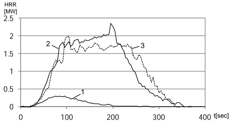
**Figure 7:** Evolution of the inferred heat release rate
