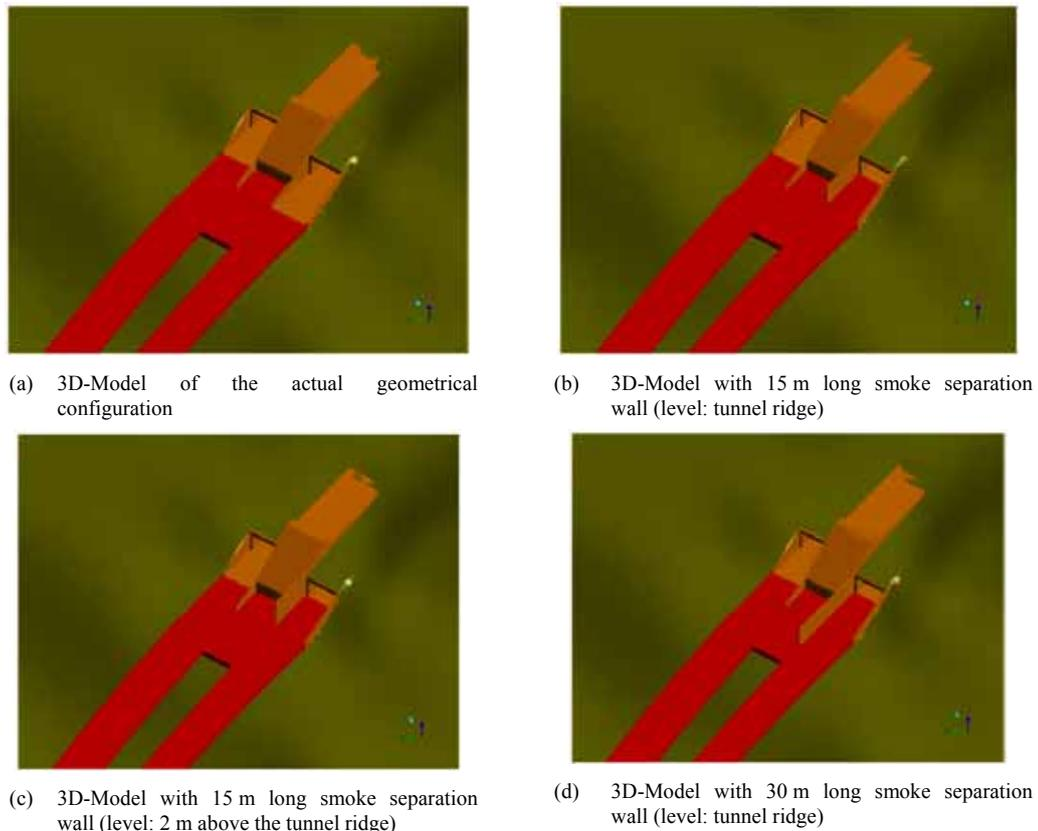
**Figure 2:** Geometrical variations used in 3-D numerical simulations
