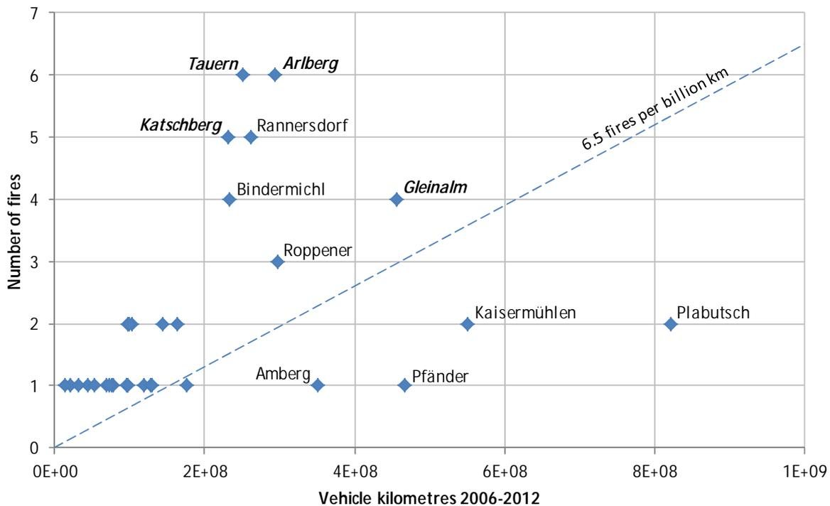
**Figure 1:** Number of fires vs. travelled vehicle kilometres in different Austrian tunnels (tunnels with long and steep approaches *in italics*)
