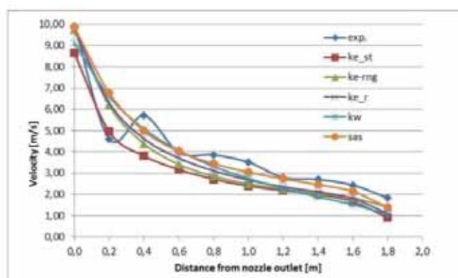
**Figure 8:** Centreline Velocity ( $\alpha=0^\circ$ ,  $U=10$  m/s)
