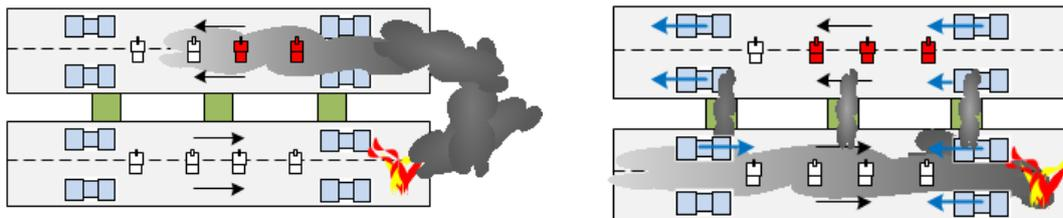
**Figure 7:** Wrong fire location detection due to portal to portal recirculation
