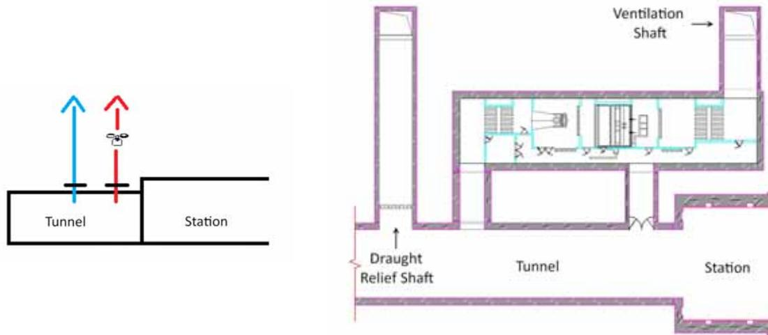
**Figure 2:** Independent draught relief and ventilation shaft
