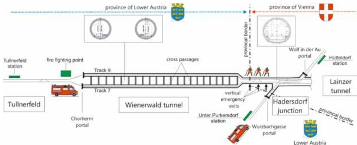
Figure 2: Change of tunnel system within the Wienerwald tunnel
