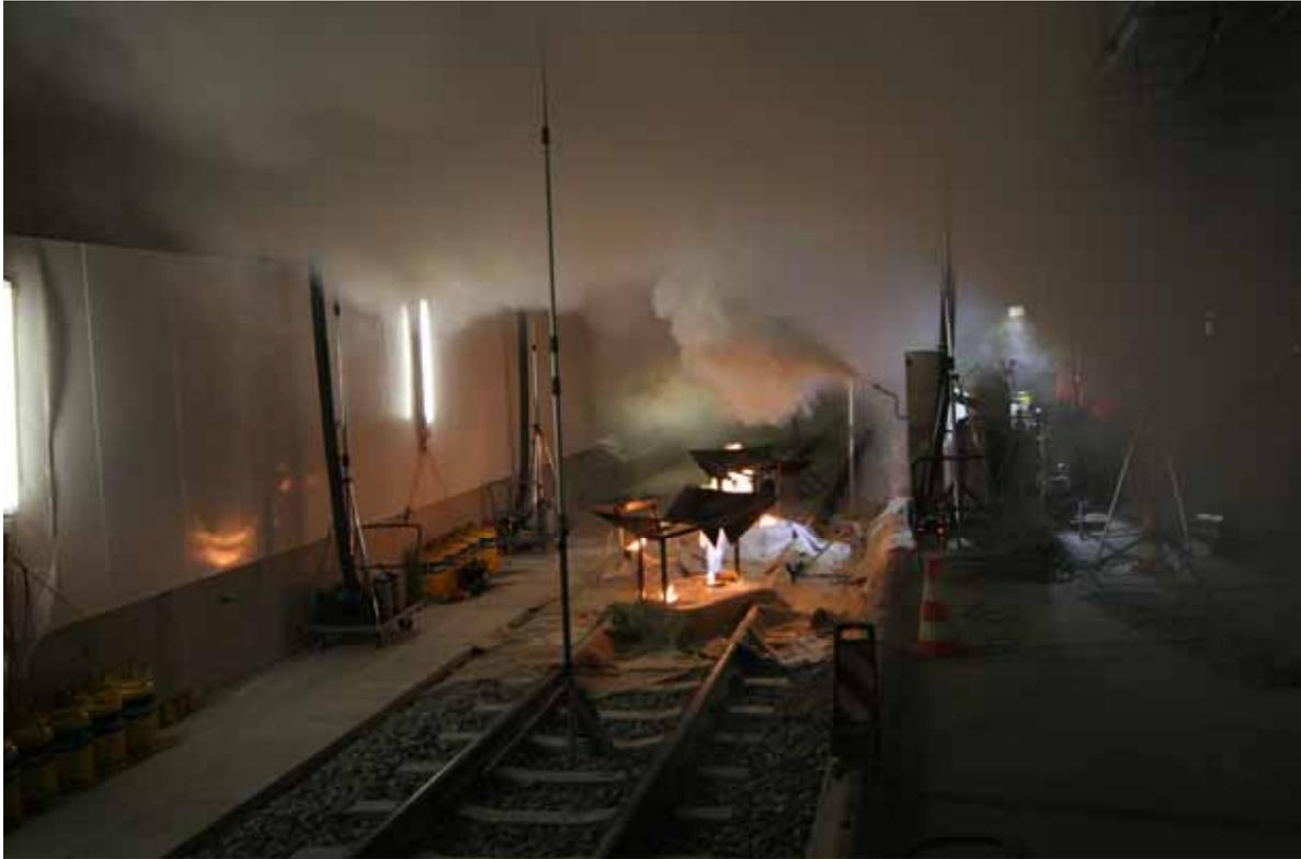
**Figure 2:** Setup of equipment for the hot smoke test
