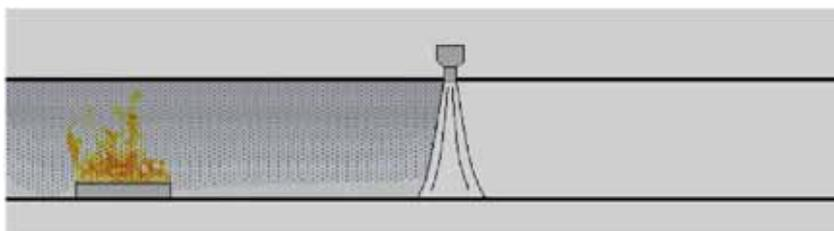
**Figure 1:** Illustration of zone separation
