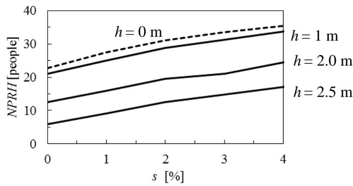
**Figure 9:** Change in *NPRH* with smoke barrier height in the case of *P10* (the dotted line is  $h = 0$  m and the solid lines are the effect of smoke barrier height)
