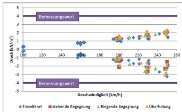
**Figure 5:** Maximum compression/suction impacts compared to the design values, Stierschweiffeldtunnel. [4]
