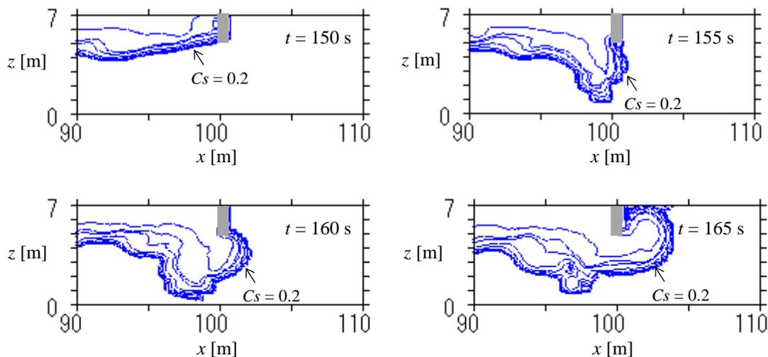
**Figure 3:** Smoke behavior close to the smoke barrier ( $h = 2$  m,  $s = 0\%$  and  $y = 0$  m).
