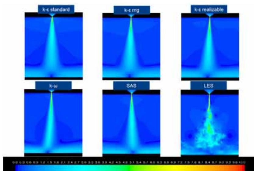
**Figure 9:** Velocity counters in cross-section of numerical domain
