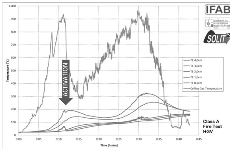
**Figure 8:** Material temperatures of a concrete specimen and ambient gas temperature
