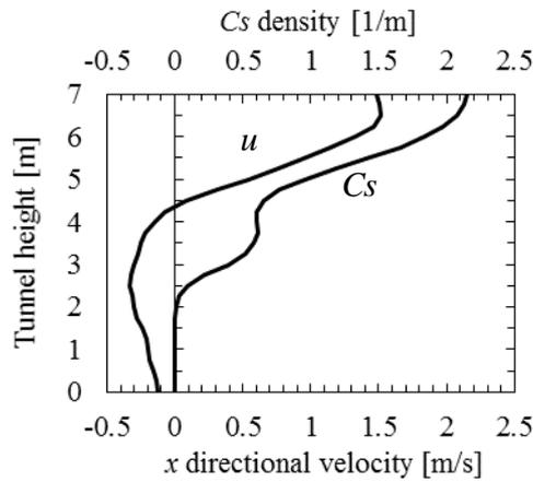
**Figure 5:** Horizontal distribution of smoke and  $x$ -direction velocity in the case of  $h = 2$  m
