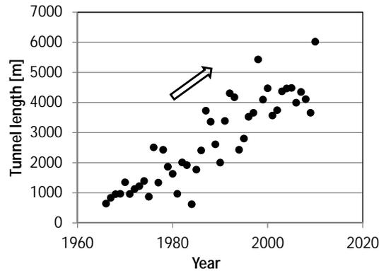
**Figure 4:** Change of maximum application length of longitudinal ventilation systems using jet fans in two-way traffic tunnels
