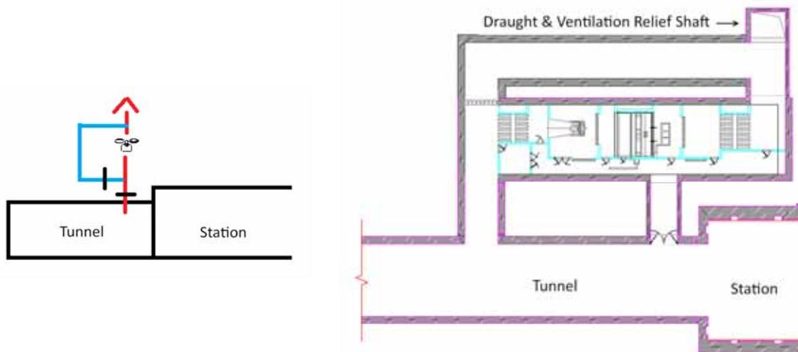
**Figure 5:** Common structural intake and exhaust shaft
