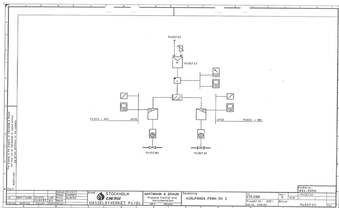
**Figure 2:** Example of an overview with graphics function blocks according to VGB-standard.
