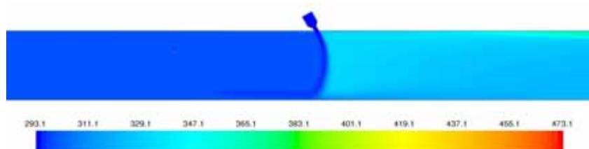
**Figure 14:** Temperature range in cross section  $e=10$  cm,  $U=10$  m/s (K)
