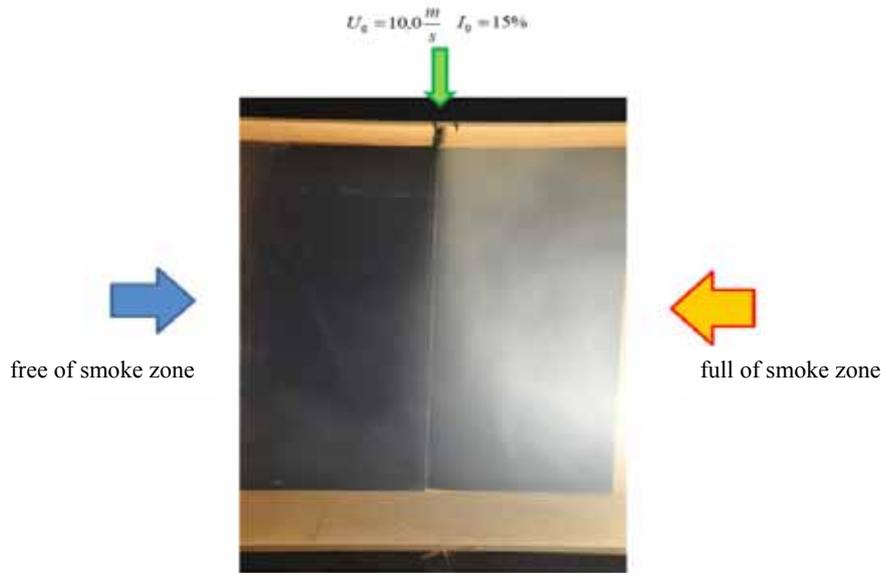
**Figure 10:** Division of two zones using air curtain
