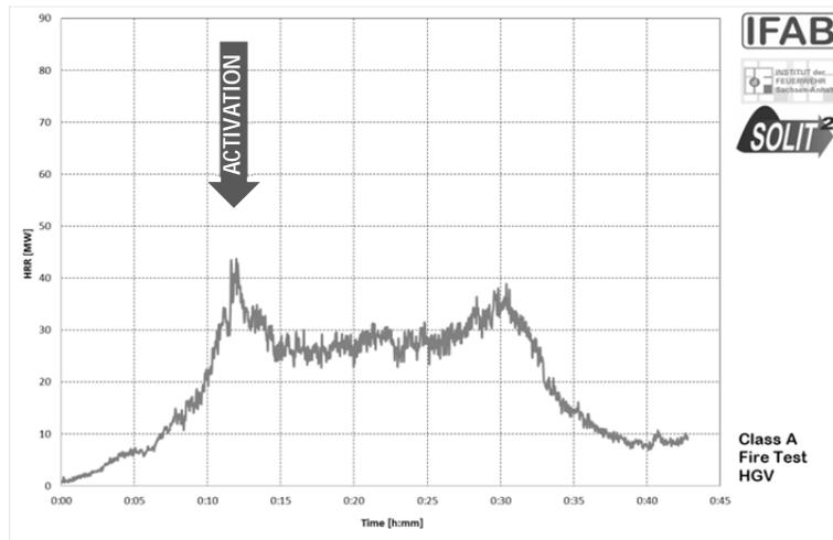
**Figure 7:** HRR during a class A fire test with activated FFFS
