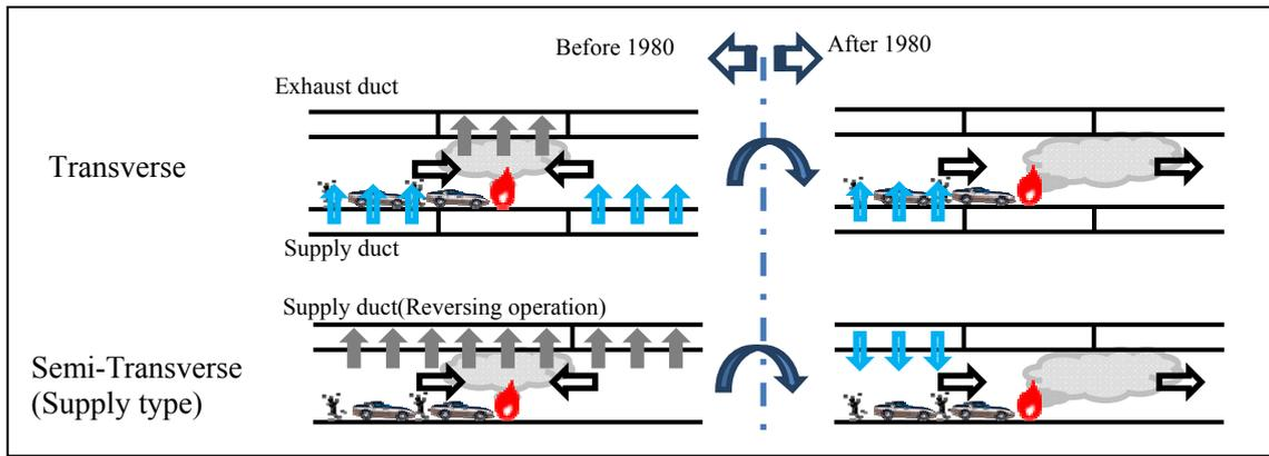
**Figure 5:** Change of smoke control of the transverse and the semi-transverse ventilation systems
