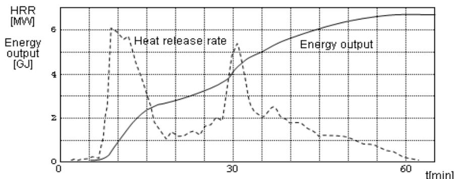
**Figure 1:** Heat release rate of plastic car fire ( EUREKA fire tests <sup>[3]</sup>)
