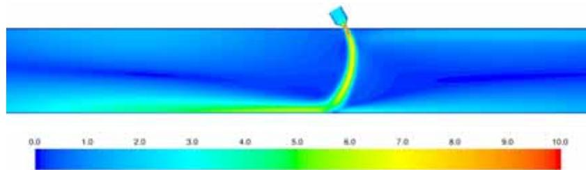
**Figure 11:** Velocity profile in cross section  $e=5$  cm,  $U= 10$  m/s
