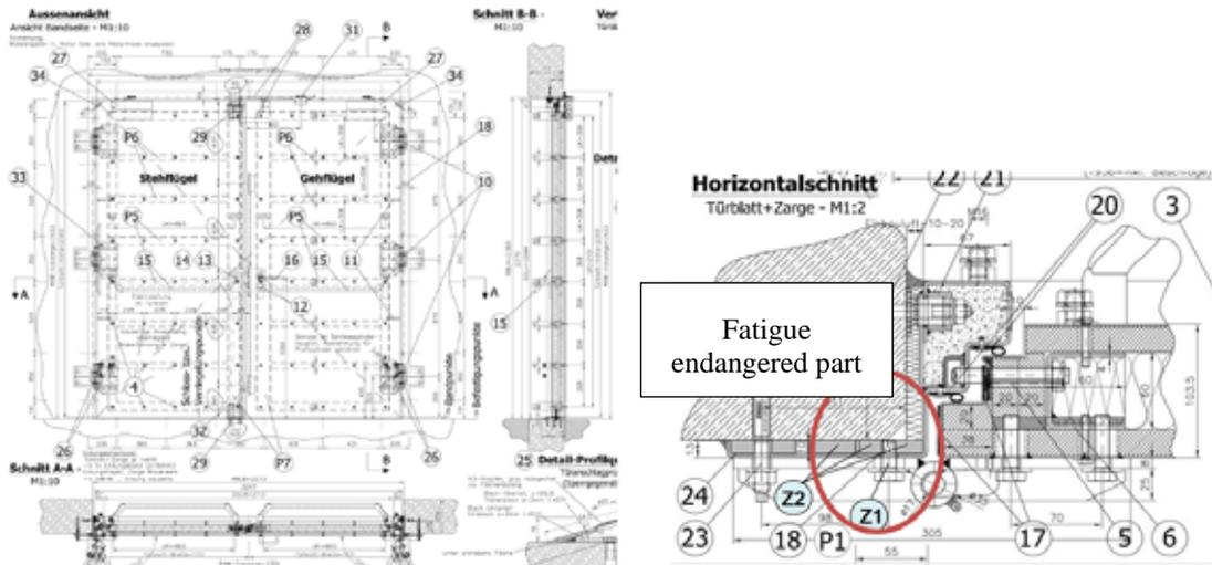
**Figure 1:** Blue prints of the emergency exit door, Detail of the attachment of the hinges to the door frames. [3]
