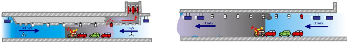
**Figure 1:** Result of wrong fire location detection: exhaust ventilation (left) and longitudinal ventilation (right)
