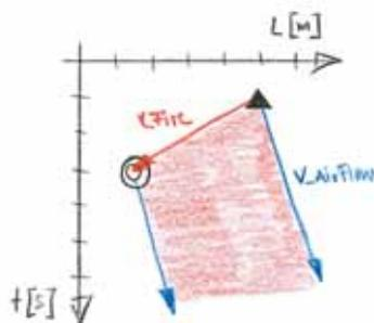
**Figure 4:** Air flow  $\rightarrow$ , Fire moving  $\leftarrow$ , constant smoke production
