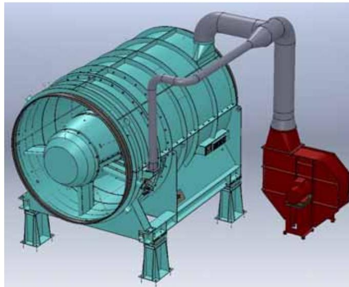
**Figure 2:** Exhaust fan with auxiliary cooling fan
