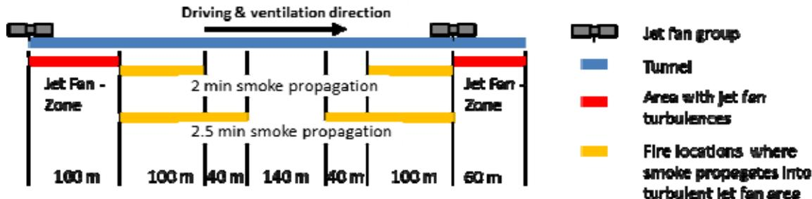
**Figure 4:** Illustration of fire locations where activation of jet fans would result in destratified smoke propagation for fan installation at portals
