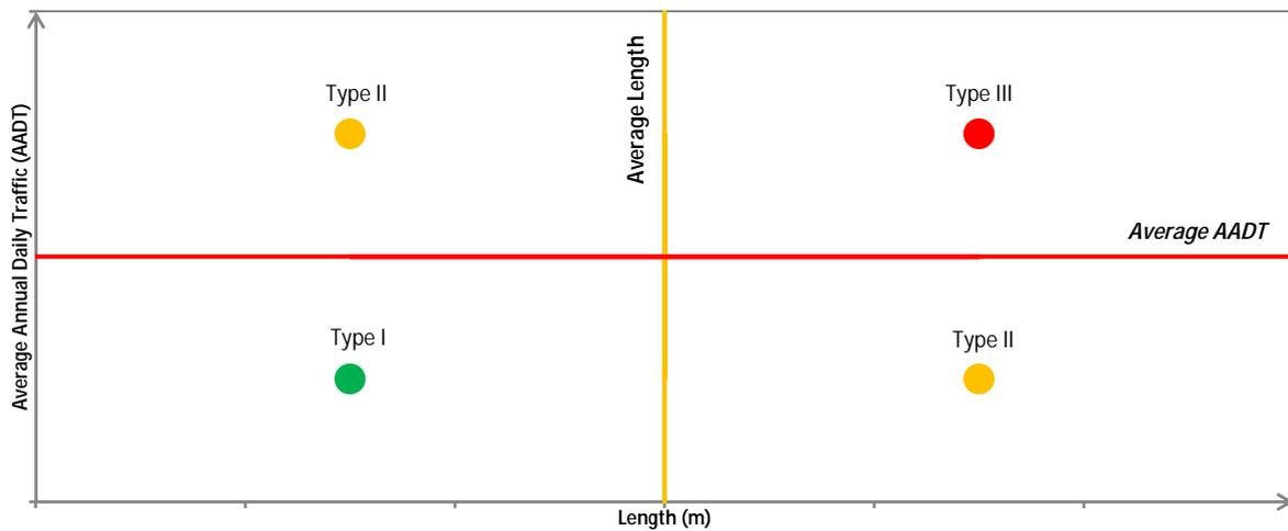
**Figure 3:** Concept for splitting road tunnels into different maintenance types
