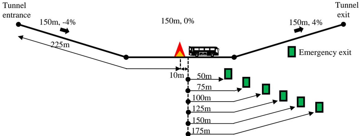
**Figure 8:** Arrangement of emergency exits [225m]
