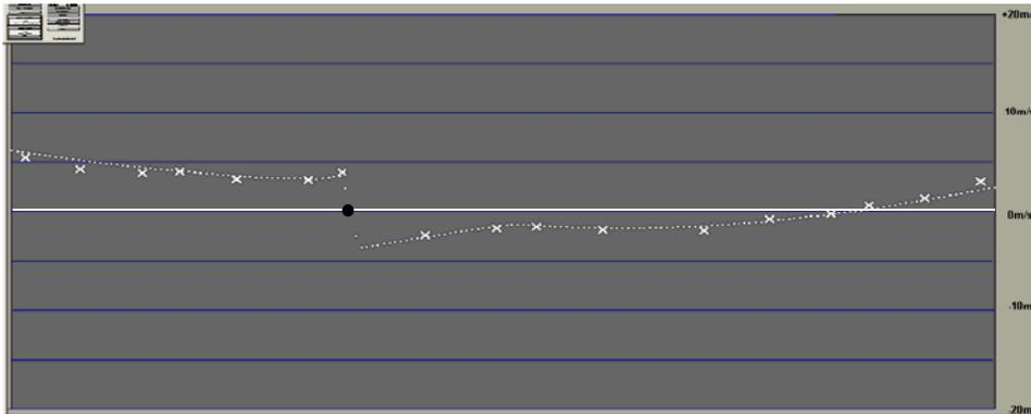
**Figure 7:** Gotthard road tunnel, theoretic calculated curve and measured values (x)
