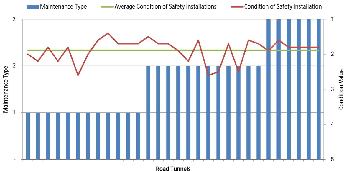
**Figure 5:** Maintenance type and condition of safety installations in road tunnels
