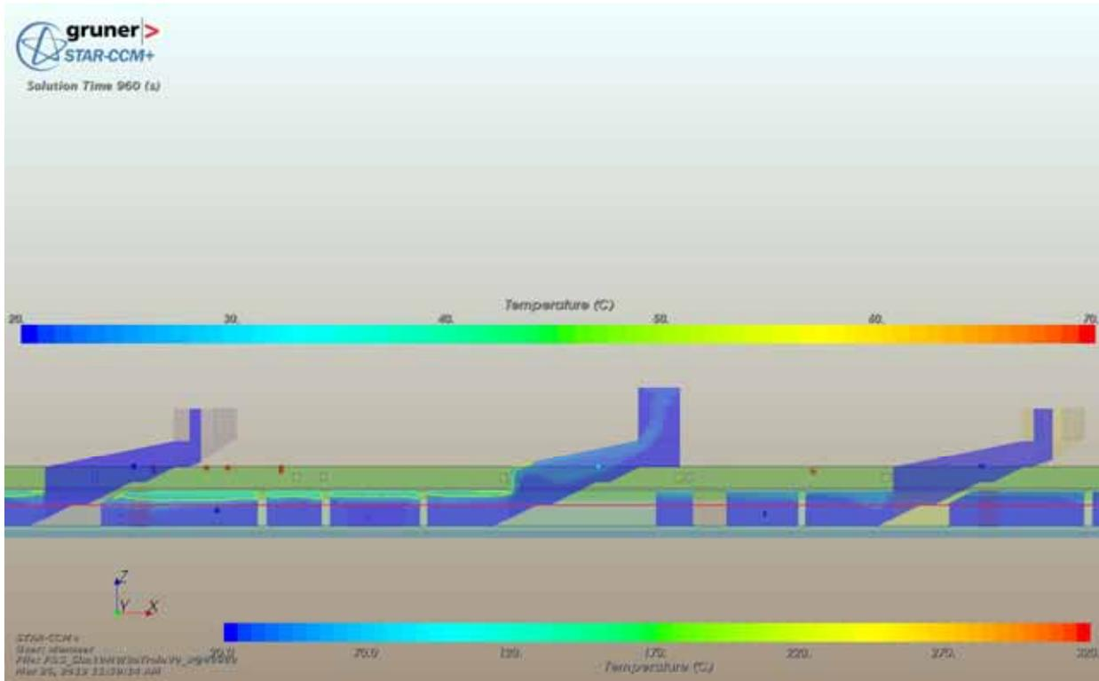
**Figure 5:** Example of compliance with the safety objective "temperature in the low-smoke layer" - longitudinal section of the station
