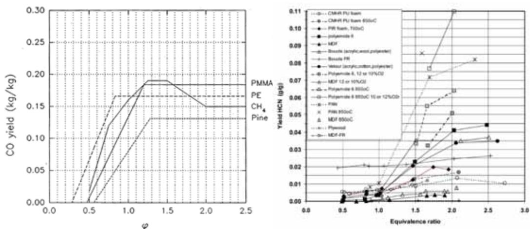
**Figure 3:** CO yield in terms of equivalence ratio measured in catcher hood experiments (Left) [4] and in the tube furnace (right) [7].
