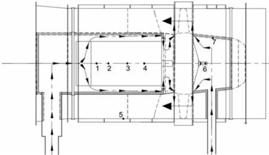
**Figure 3:** Cooling air flow with auxiliary cooling fan
