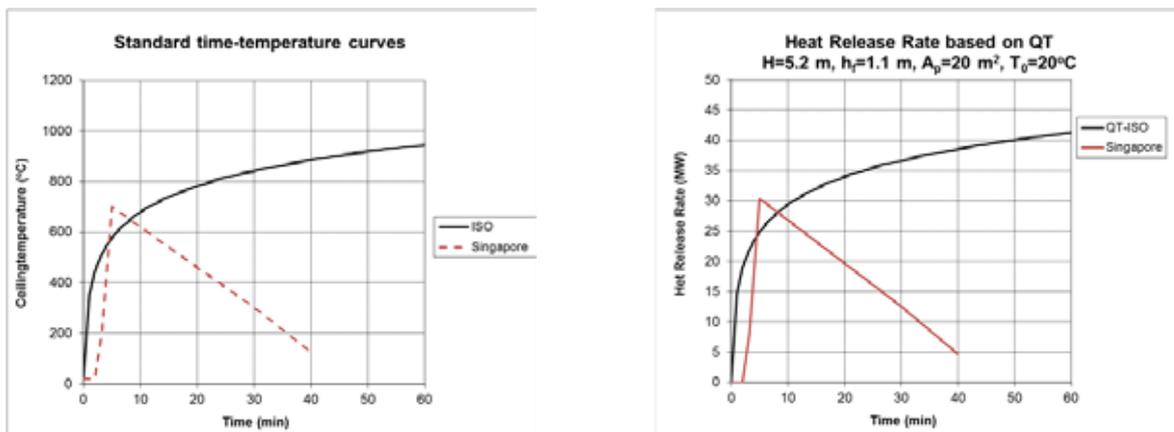
**Figure 3:** The Singapore time-temperature curve (left) and corresponding total HRR calculated for the Singapore tests using equation (3) (right).
