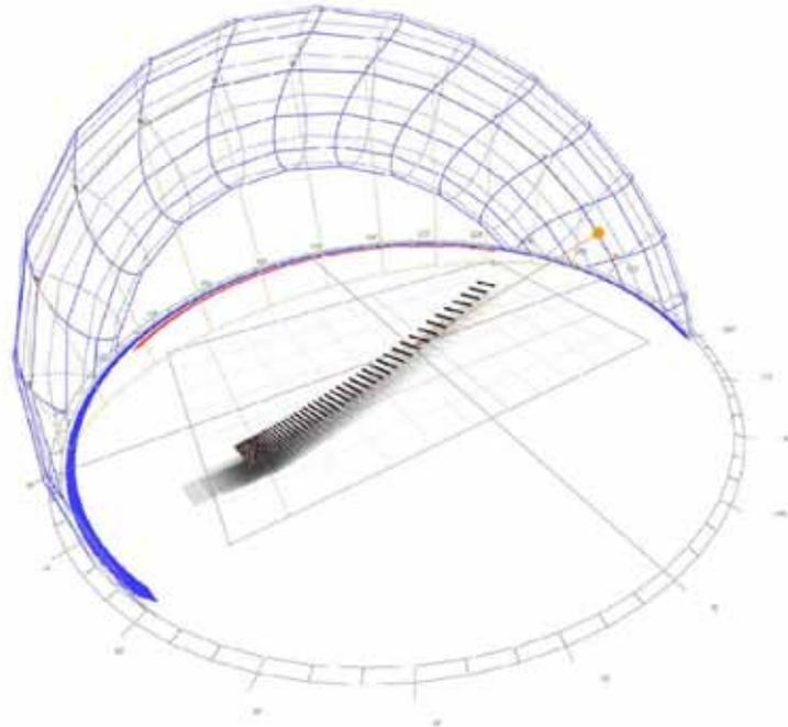
**Figure 3:** Map of solar trajectories and projected shadows
