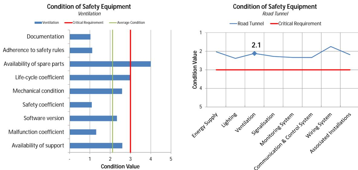
**Figure 1:** Specimen illustration of a ventilation system's condition assessment and its integration into the overall picture of a tunnel's safety equipment condition
