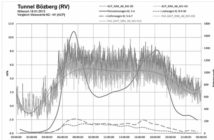
**Figure 3:** Tunnel Bözberg, air speed and traffic data.
