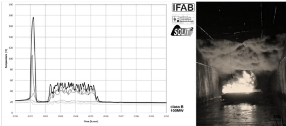
**Figure 5:** Temperatures 15 m upstream due to “Back layering” during a 100 MW class B fire test
