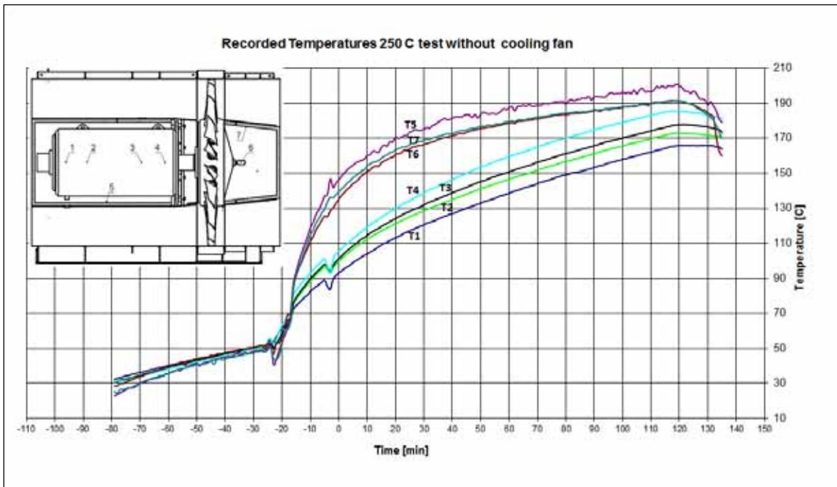
Figure 6: Recorded temperatures, test at 250 °C without cooling fan
