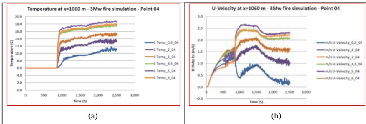
**Fig. 6:** Temperature (a), U-velocity (b) at tunnel cross section 04, 3MW case
