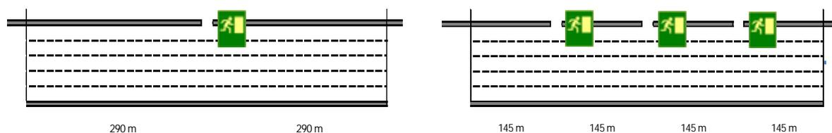
**Figure 1:** Illustration of 5 lane tunnel layout for 1 and 3 cross-passages
