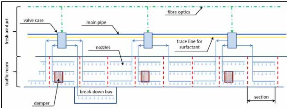
**Figure 14:** Scheme of the high pressure water mist system.
