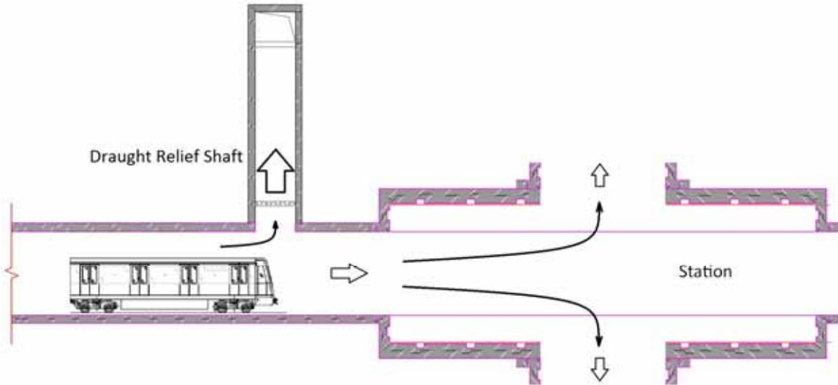
**Figure 1:** Air blast flows in a station
