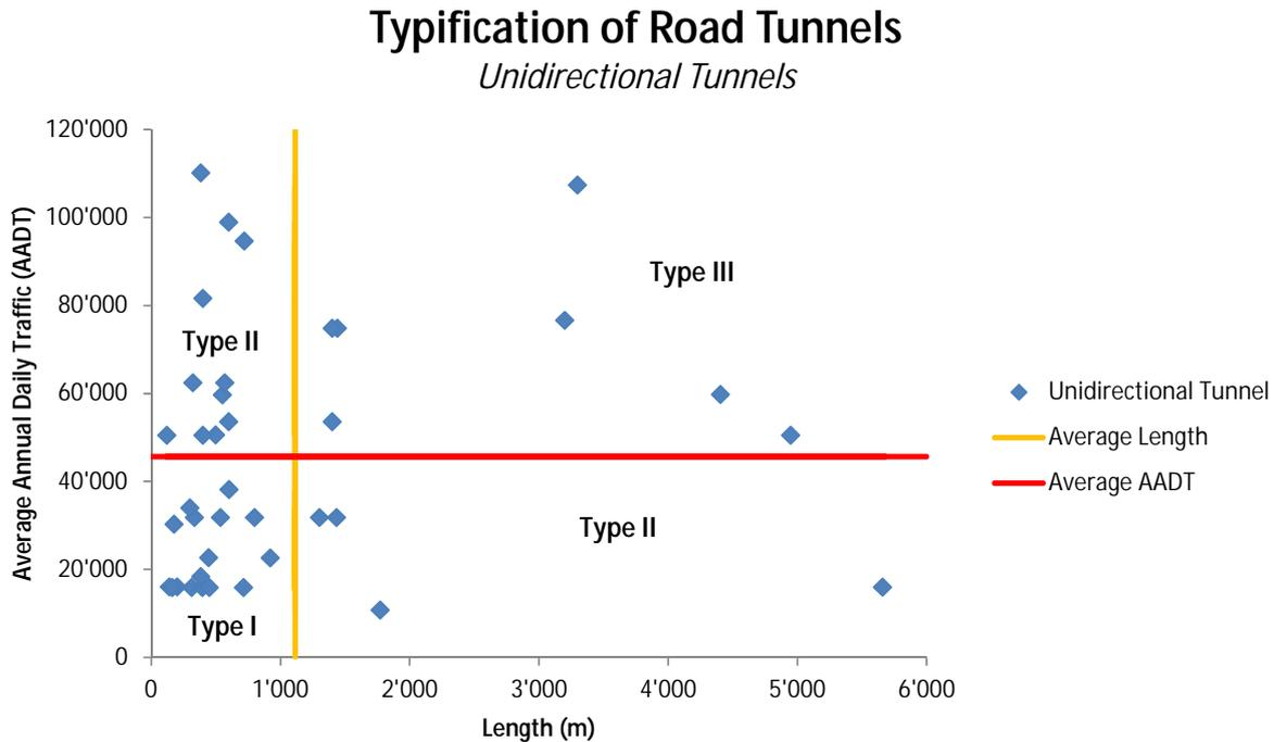
**Figure 4:** Typification of unidirectional road tunnels
