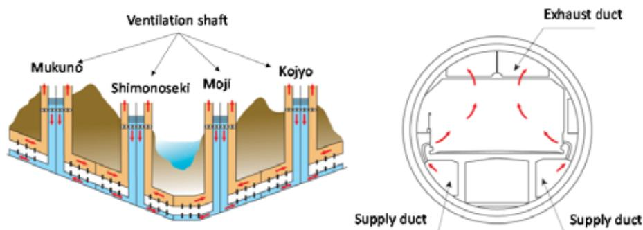
**Figure 1:** Schematic view of the ventilation system in the Kanmon Tunnel
