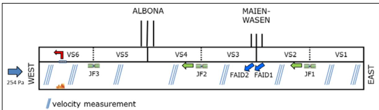
**Figure 12:** Fire ventilation for an incident in ventilation section VS6.
