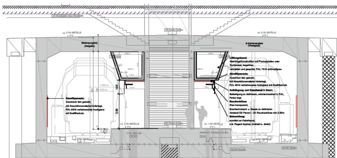
**Figure 1:** Cross-section of "Luzern Allmend/Messe" station with extraction duct
