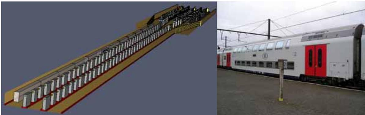
**Figure 6:** CFD model tunnel and station (Left) and Double-decker railway-car (Right) [15].
