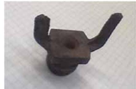
**Figure 4:** Damaged sprinkler - Brass made sprinkler nozzle
