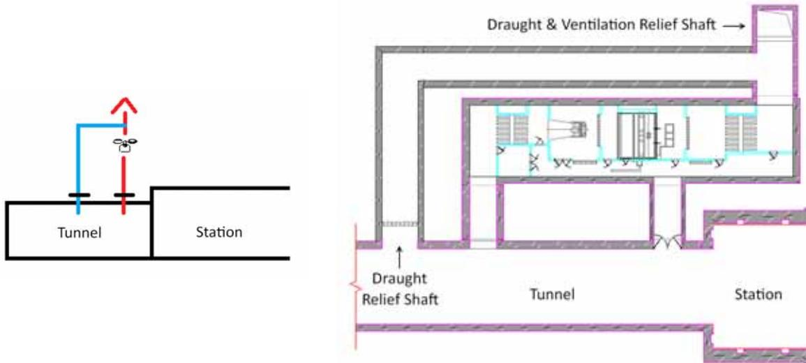
**Figure 4:** Common structural exhaust and ventilation shaft with different intake shaft
