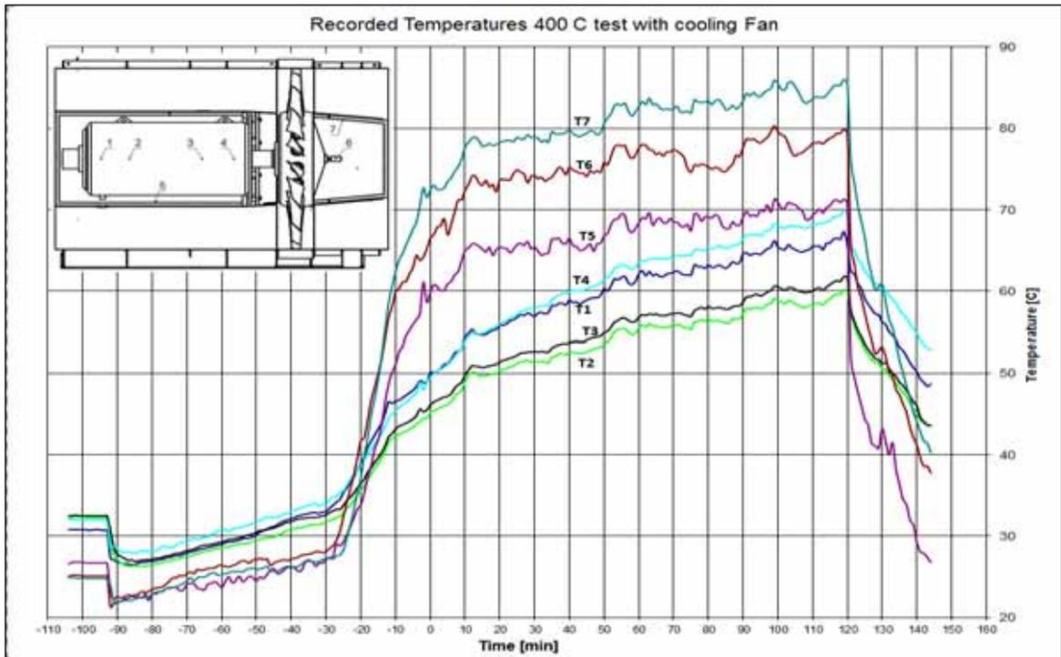
Figure 5: Recorded temperatures, test at 400 °C with cooling fan
