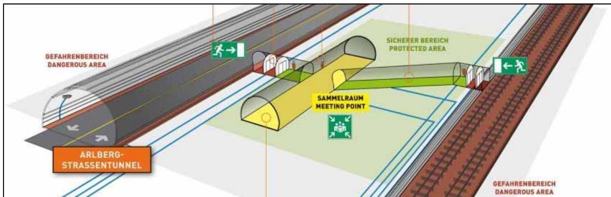
**Figure 3:** Example of an egress way in Arlberg road tunnel (ASFINAG).
