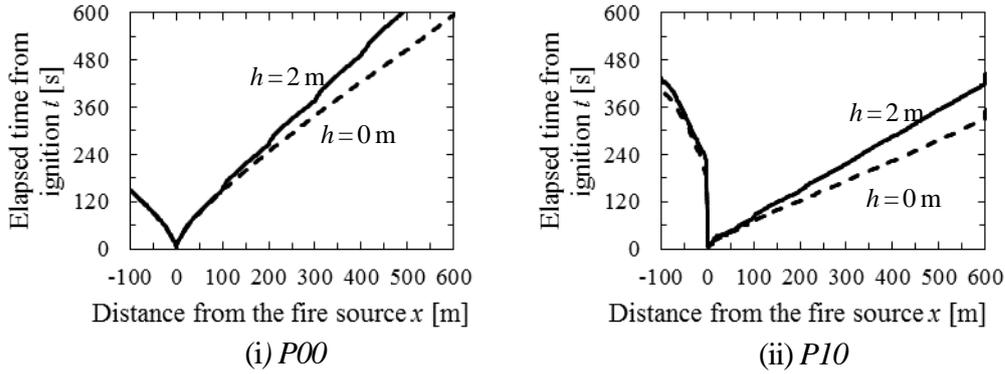
**Figure 4:** Comparison of cases without smoke barriers ( $h = 0$  m) and with smoke barriers ( $h = 2$  m) for difference in location of smoke tip ( $x - t$  distribution,  $s = 0\%$  and averaged width direction, the dotted line is  $h = 0$  m and the solid lines are the effect of smoke barrier height  $h$ )
