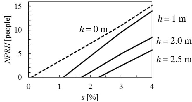
**Figure 8:** Change in *NPRH* with smoke barrier height in the case of *P00* (the dotted line is  $h = 0$  m and the solid lines are the effect of smoke barrier height)
