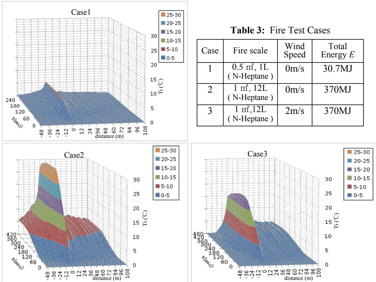
Figure 3: Temperature increases in Space and Time,  $T \{ x, t \}$
