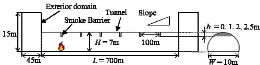
**Figure 2:** Dimensions of the model tunnel and computational domains.
