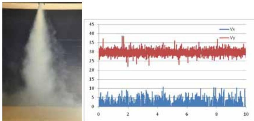
**Figure 6:** Velocity at the nozzle outlet
