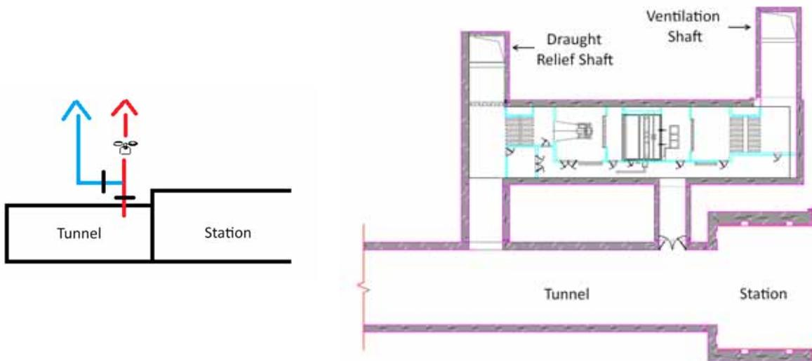
**Figure 3:** Common intake shaft for draught relief and different in exhaust shaft
